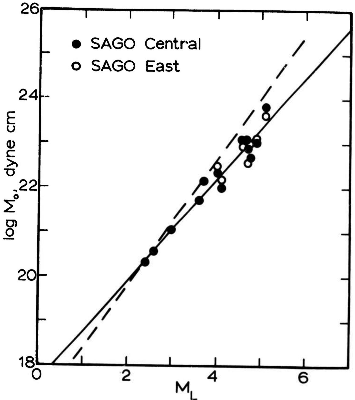
Figure 7. Relation between seismic moment and magnitude. The solid line was fit to the data points by linear regression and the dashed line is from Wyss and Brune (1968). The SAGO-East values have been divided by a factor of 3 to remove an amplification effect.
