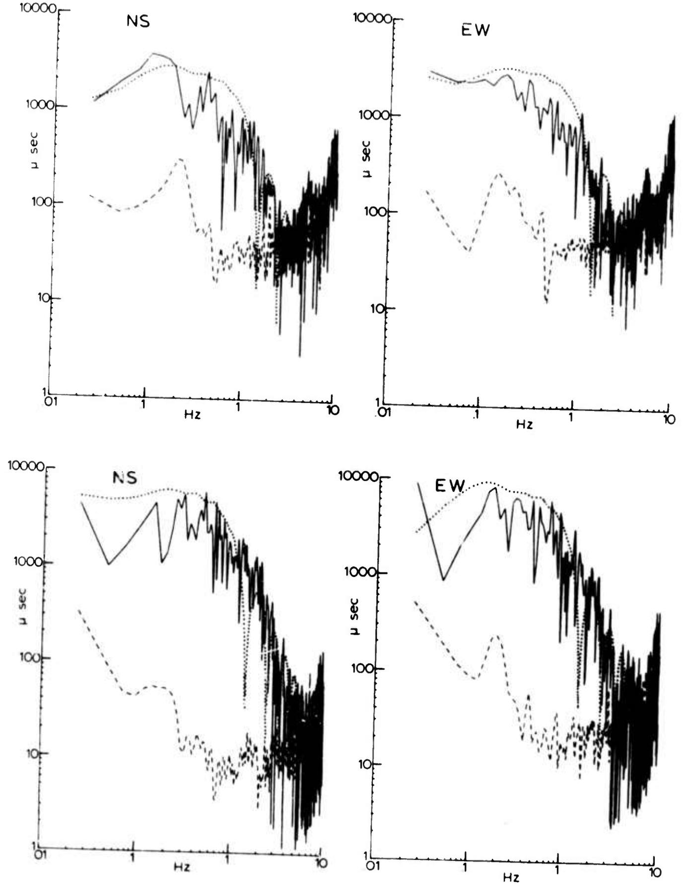
Figure 20. Amplitude density spectra calculated for event 4a (Table 1) from seismograms (Figure 19) recorded at SAGO-Central (top 2 spectra) and at SAGO-East (bottom 2 spectra). The solid lines are calculated from the observed seismograms, the dashed lines are estimates of the noise, and the dotted lines are calculated from the synthetic seismograms
