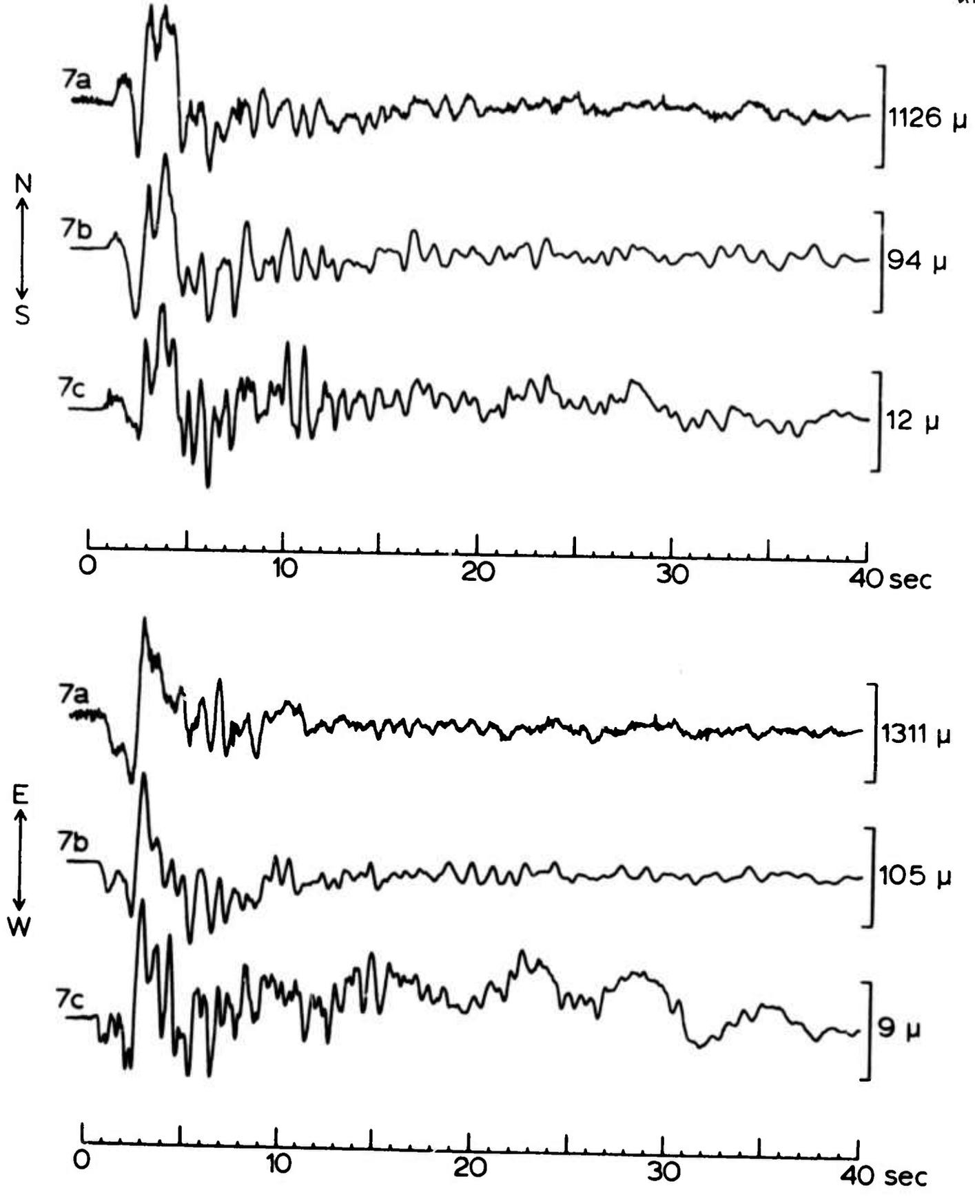
Figure 18. The displacement seismograms recorded at SAGO-Central from event 7a, 7b, and 7c (Table 1) with magnitudes 4.9, 4.1, and 3.0, respectively.
