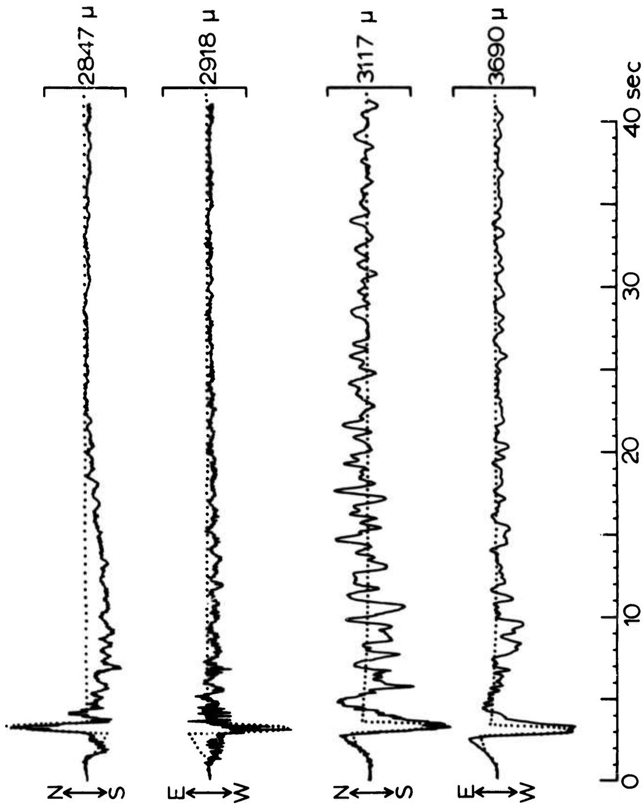
Figure 9. The displacement seismograms (solid lines) from event 1 (Table 1) recorded at SAGO-Central (top 2 traces) and at SAGO-East (bottom 2 traces). The dotted lines are synthetic seismograms calculated for this earthquake.
