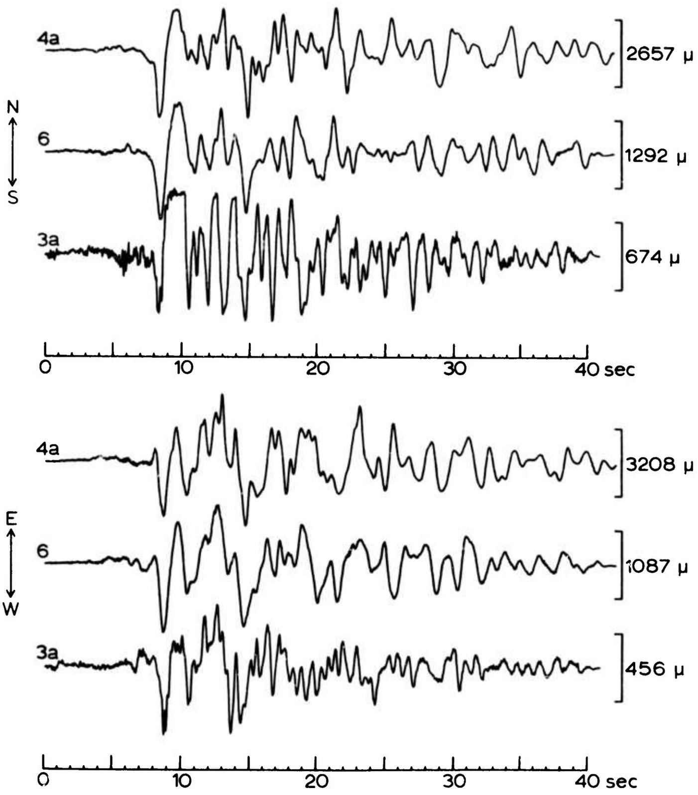
Figure 21. The displacement seismograms recorded at SAGO-East from events 4a, 6, and 3a (Table 1) at epicentral distances of 31, 22, and 15 km, respectively. The seismograms have been aligned for coincidence of the S pulse at about 8 sec.
