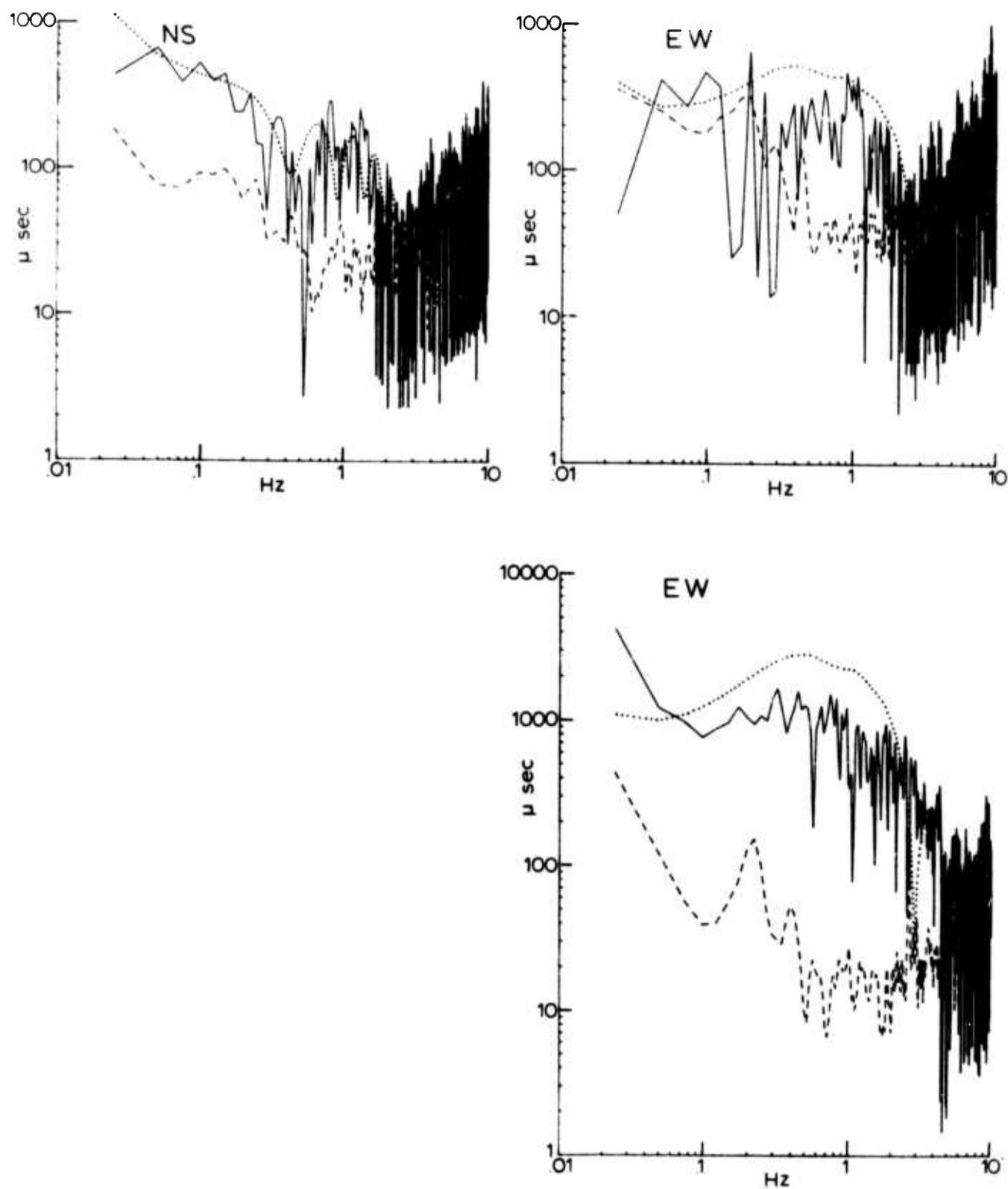
Figure 15. Amplitude density spectra calculated for event 2 (Table 1) from seismograms (Figure 14) recorded at SAGO-Central (top 2 spectra) and at SAGO-East (bottom spectrum). The solid lines are calculated from the observed seismograms, the dashed lines are estimates of the noise, and the dotted lines are calculated from the synthetic seismograms.
