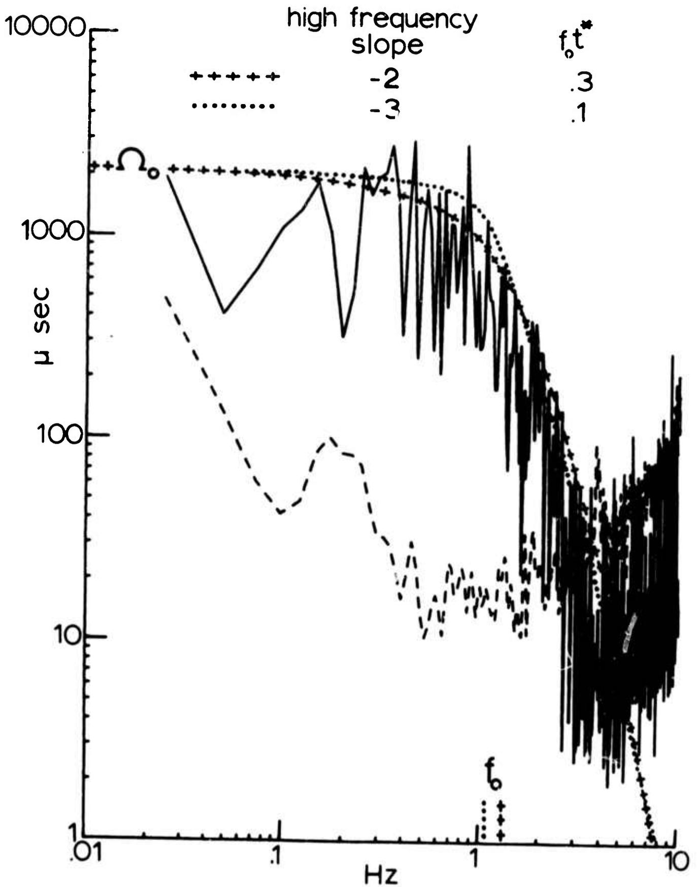
Figure 6. Example illustrating two different estimates of the low-frequency level  $\Omega_0$  and the corner frequency  $f_c$  of the spectrum from the NS component at SAGO-East from event 6 (Table 1).
