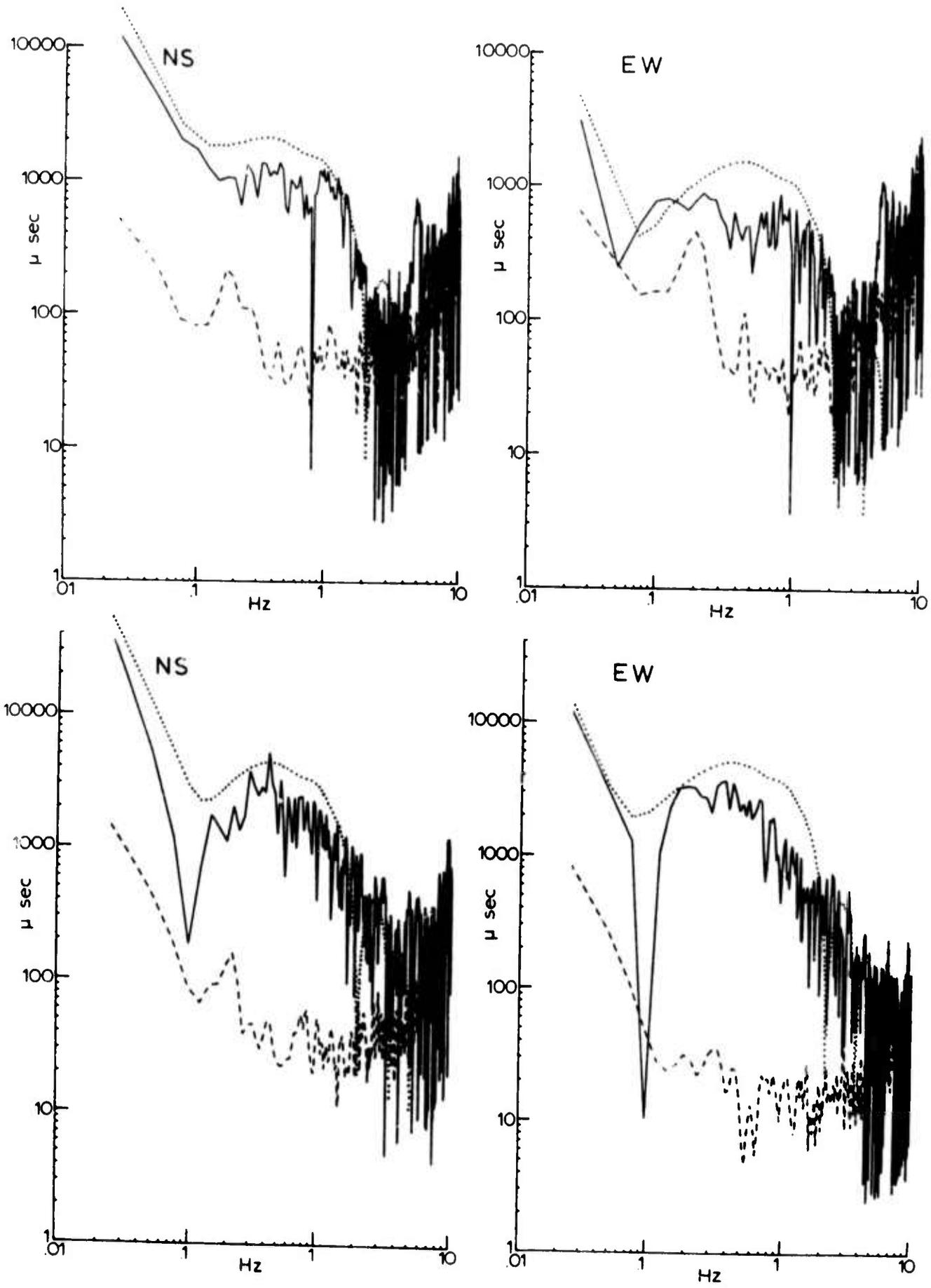
Figure 13. Amplitude density spectra calculated for event 1 (Table 1). The solid and dashed lines are identical to those of Figure 10 but the dotted lines are calculated from the synthetic seismograms of Figure 12 which include the effects of an impulse in tilt.
