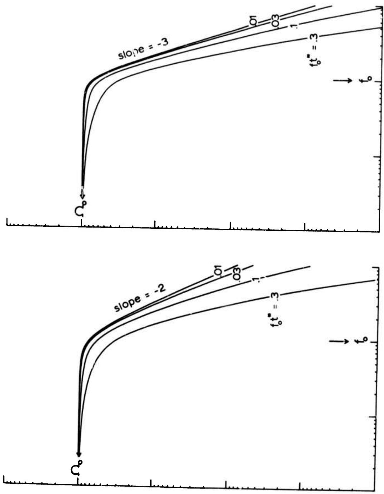
Figure 5. Templates used to obtain spectral estimates of the low-frequency level  $\Omega_0$  and the corner frequency  $f_0$  for the cases where the high-frequency slope is -2 (left) and -3 (right) and for four values of  $t^*$ .
