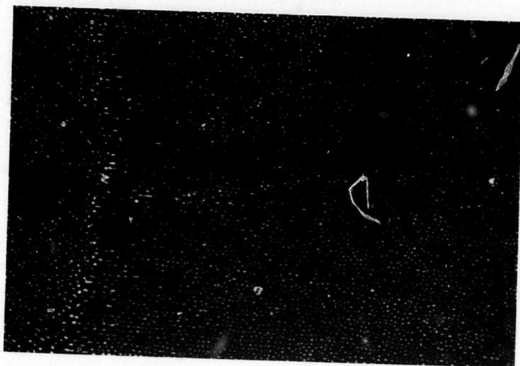
Figure II-6.  $\text{CeO}_2$  Doped  $\text{Gd}_2\text{O}_3$ -Mo Sample Grown at 4 cm/hr Displaying Mo Fibers in the Cell Interior Which Gradually Grade to Platelets at the Cell Boundary. Dark Field, X600.
