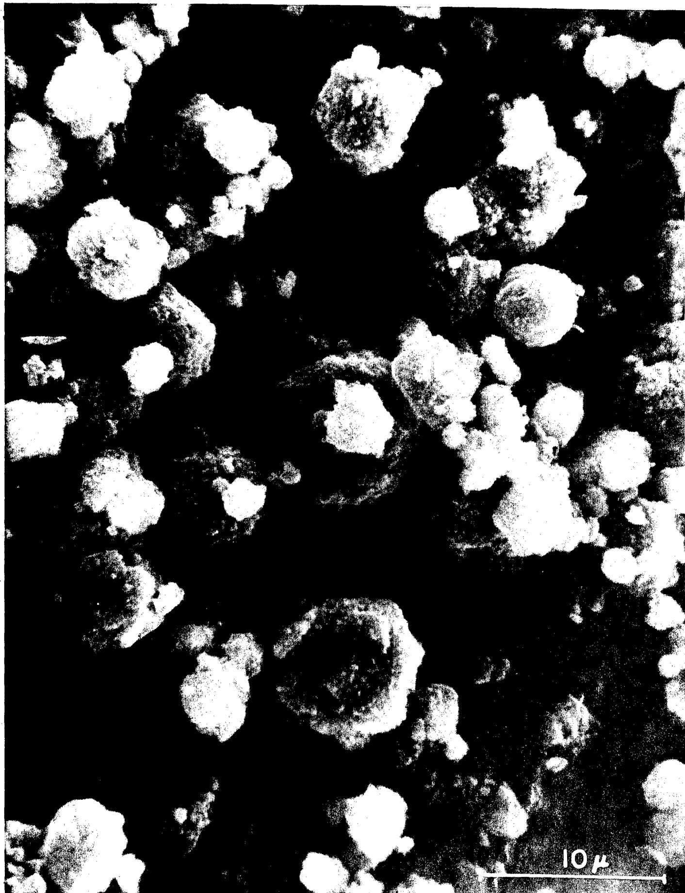
Figure 2. SCANNING ELECTRON PHOTOMICROGRAPH OF "BeO EXHAUST PRODUCT". x 5000
