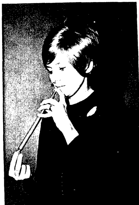
Figure 3. AFTER THE DISTAL CAP IS SECURE, THE PROXIMAL END OF THE PIPETTE IS REMOVED FROM THE MOUTH AND QUICKLY SEALED WITH A FINGER TIP.
