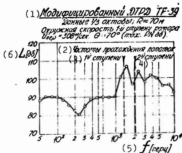
Fig. 16. The compressor noise spectrum of a DTRD with y \sim 5 .
