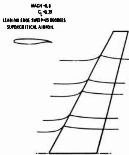
Figure 30. Streamline pattern on high speed wing
