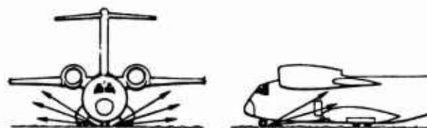
Figure 26. Overwing engines - effect on inlet ingestion
