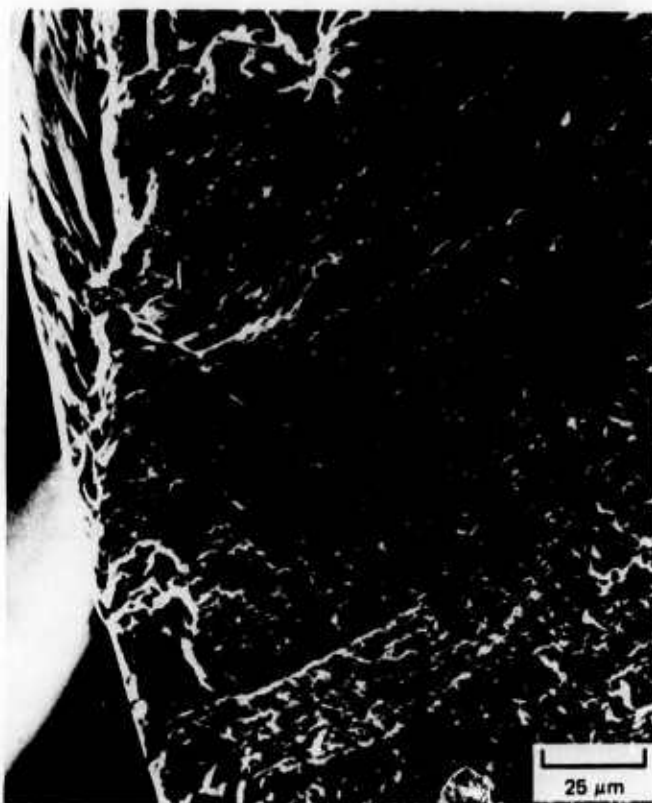
Fig. 12 — Beach markings of a fatigue crack in a type-B wire of a titanium wire rope that was fatigue tested (Fig. 11)
