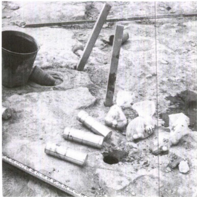
Figure 2.13 Artificial missiles (cylinder packages and sphere packages) prior to emplacement in NX-size boreholes.
