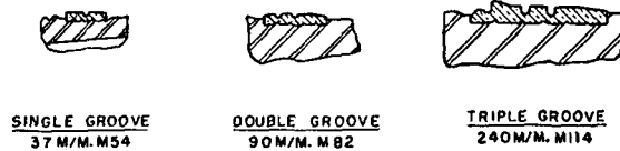
TYPES OF ROTATING BANDS FOR ARTILLERY PROJECTILES
