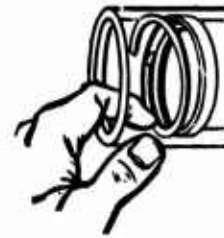
c. INSTALLATION OF "T" SEAL SPLIT BACKUP RINGS
