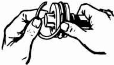
c. INSTALLATION OF "T" SEAL SPLIT BACKUP RINGS
