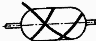
Fig. 71. Helical crossover winding
