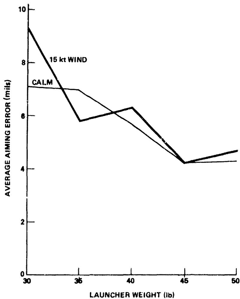
Figure 4. Average Aiming Error at Uncoage as a Function of Weight:
