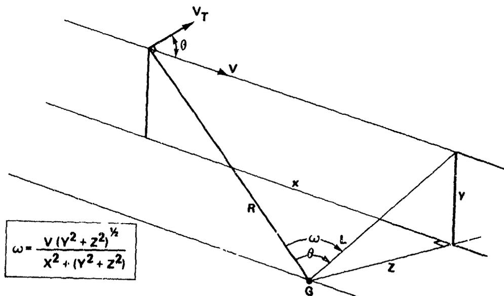
Figure A-1. Level Flight With/Without Offset
