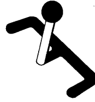
FIGURE 8-5. One method of preventing accidental activation is by requiring sequential application of force in at least two directions.
