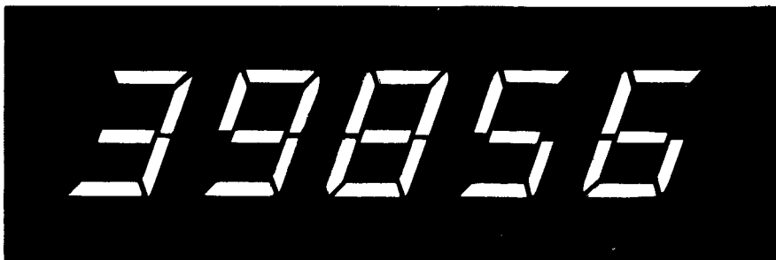
FIGURE 3-73. Seven-stroke segment display format of numeric symbols (Fuller, 1965).
