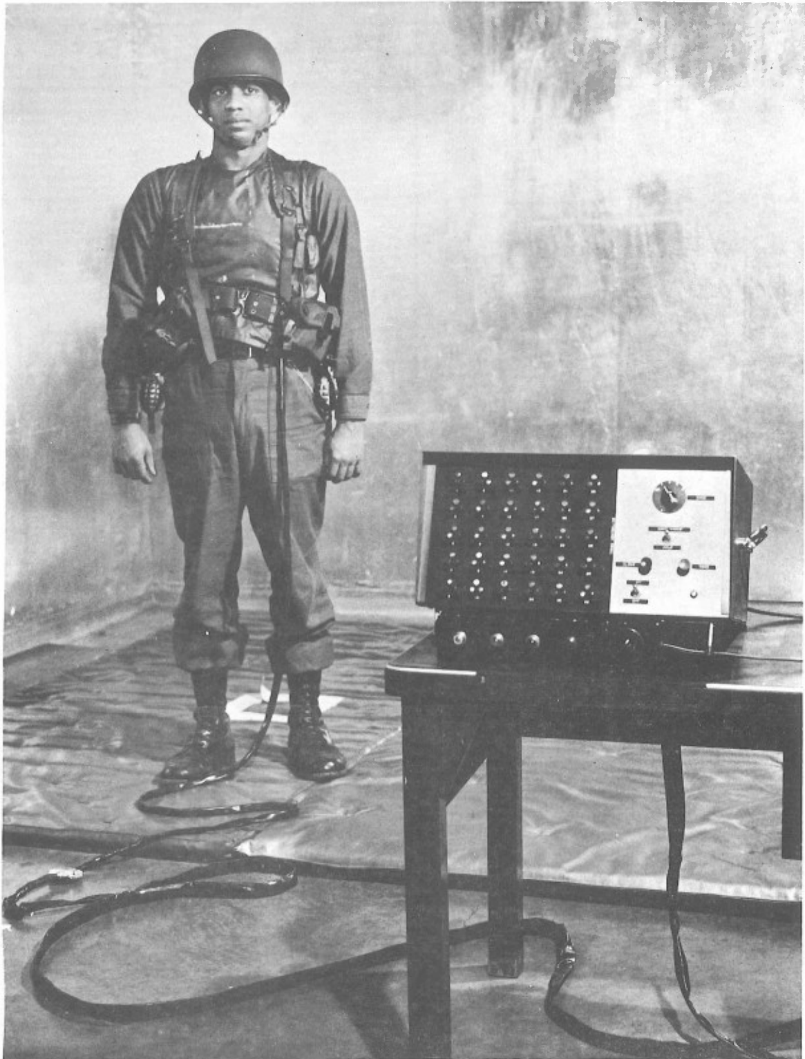
Figure 14. LCE worn over the Sensor Garment, and connected with the Load Distribution Analyzer.
