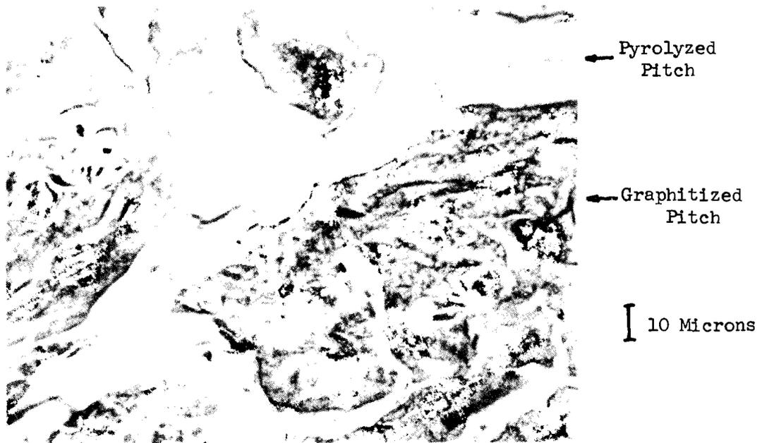
Figure 20. Photomicrograph of Multidirectional Composite After Two Impregnations and Pyrolysis - Graphitization - Three Impregnations
