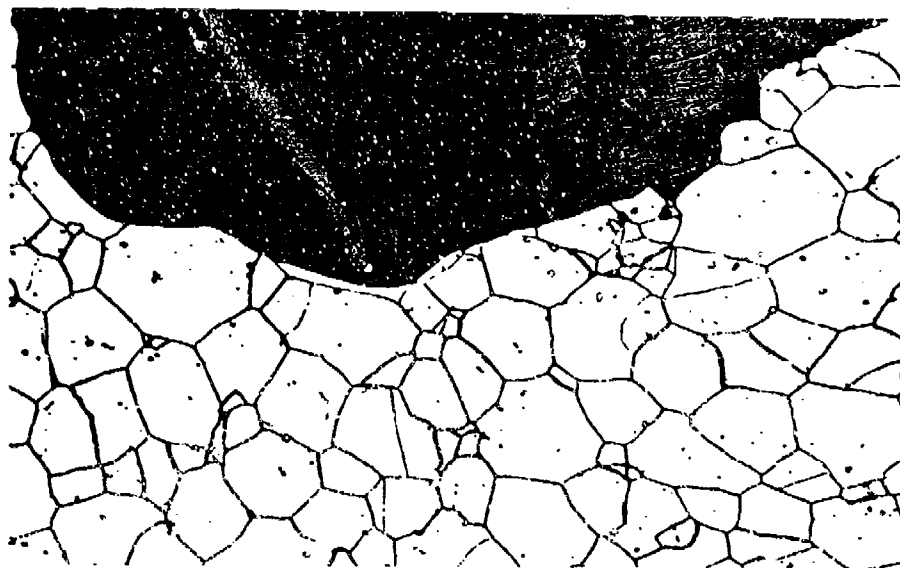
FIGURE 83 TRANSVERSE SECTION AT 17 1/2 INCHES FROM THE CHAMBER OF A CHROME-PLATED CG-27 ALLOY BARREL AFTER FIRING 7,324 ROUNDS AND BEING DECLARED UNSERVICEABLE.
