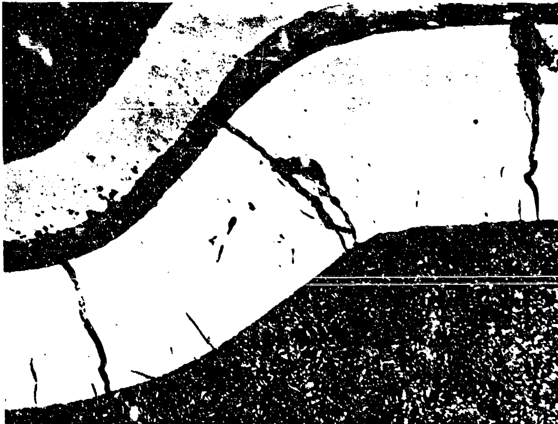
FIGURE 11 PHOTOMICROGRAPH REVEALING THE TRANSVERSE STRUCTURE ALONG THE BORE SURFACE OF A CHROMIUM-PLATED RIFLED INSERT AFTER 5 VENTED BOMB SHOTS WITH IMR PROPELLANT.
