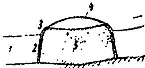
Fig. 23. Diagram of the propagation of three-dimensional detonation configurations. 1 - initiating shock wave; 2 - detonation of a shock-compressed mixture; 3 - segment of inflammation on the shock front; 4 - re-formed shock wave without inflammation; 5 - detonation products.
