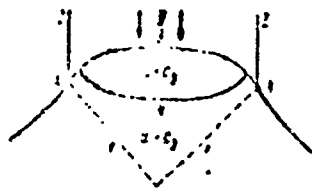
Fig. 71. Simplified scheme of the flows during stationary detonation in a charge of finite diameter. 1 - Mach lines; 2 - boundary of the charge; 3-- shock front; 4 - sound surface.
