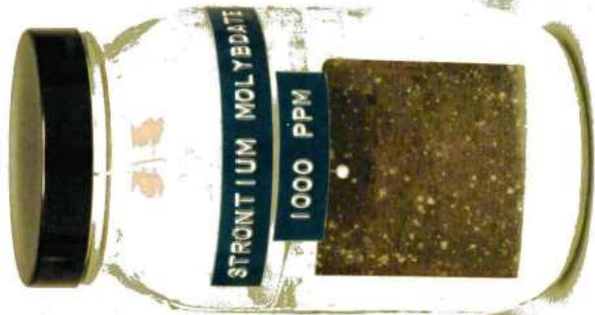
Figure 3. - 7075-Aluminum Alloy Specimen Suspended in 5% Salt Solution Containing 0.1% Inhibitor
