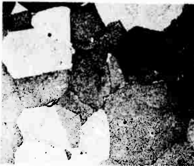
Figure 6. IN-100, low carbon, R.E.P. powder, -35 mesh. HIP @ 2275°F, 28,300 psi, 2 hrs. As pressed. Etched. 100X.
