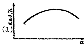
Fig. 18. Graph of steam boiler efficiency as a function of the excess air factor \alpha (at constant load).
