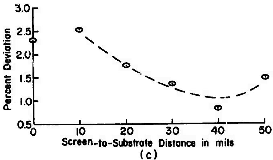
Figure 8. Effect of Screen Printer Parameters on Film Weight Deposited
