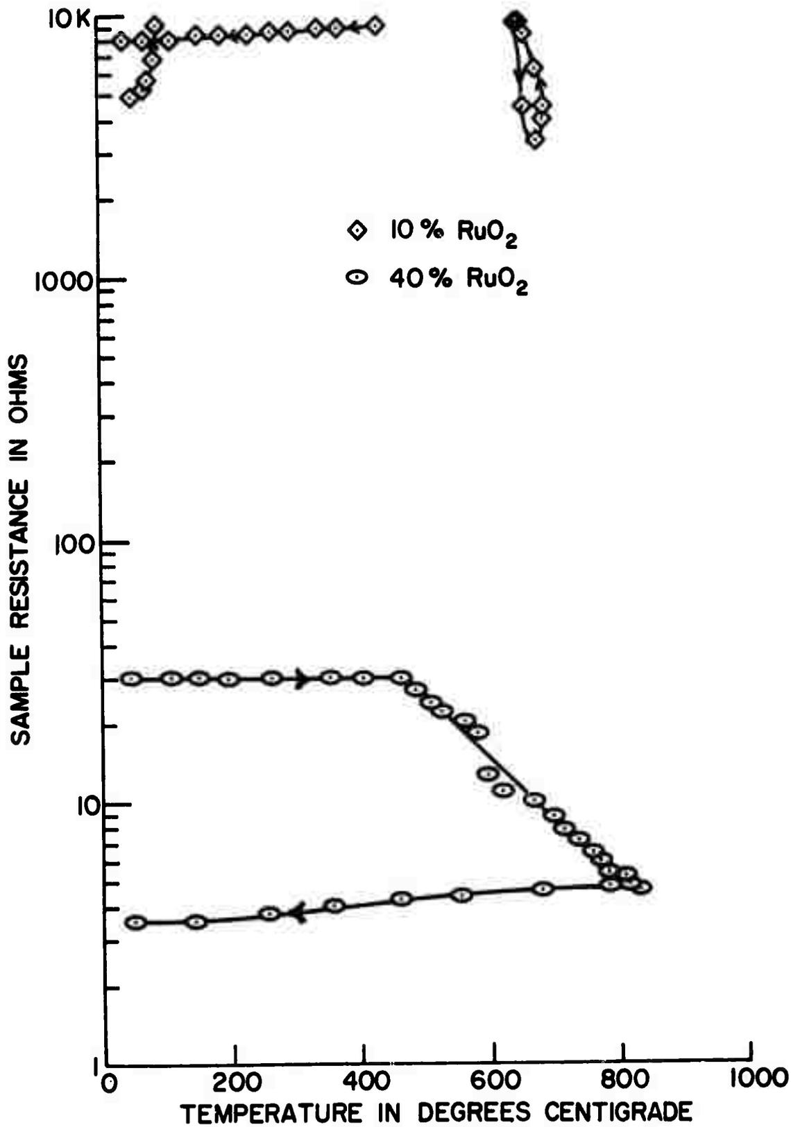
Figure 4. Resistance Changes During Thick Film Resistor Firing
