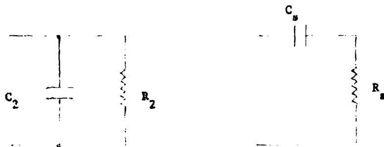
Fig 18- Equivalence between parallel combination and series combination of capacitance and resistance
