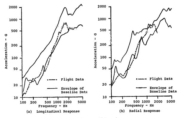
) igure 2 - Comparison of 1 light and Test Data at Pase of Attach Fitting
