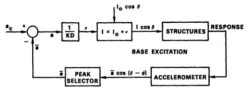
Fig. 1 - Notch control system block diagram
