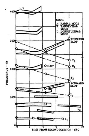
Figure 7 Modal Frequencies Measured During Acoustic Tests Compared with Vibration Data Envelope
