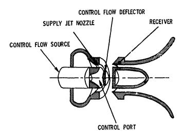
Fig. 4 - Annular Slot Jet Amplifier
