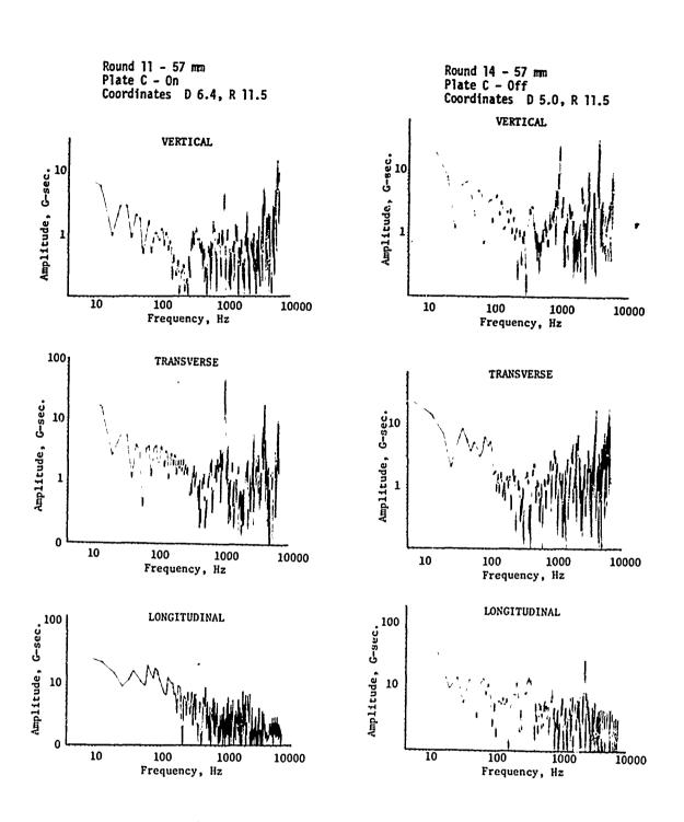
Fig. 14 - Fourier spectra from six accelerometer traces
