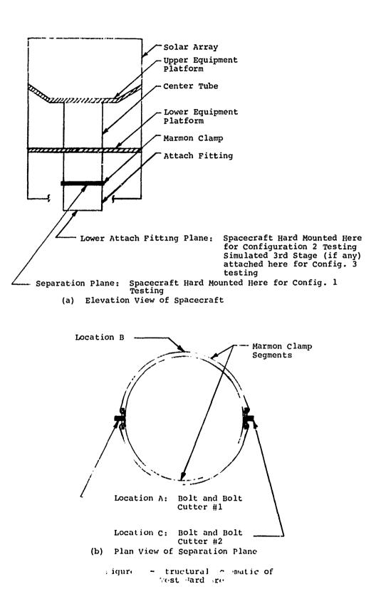
spacecraft to ground. For tests in this configuration the IMP-I lifting sling was attached to the spacecraft but did not support any weight.
