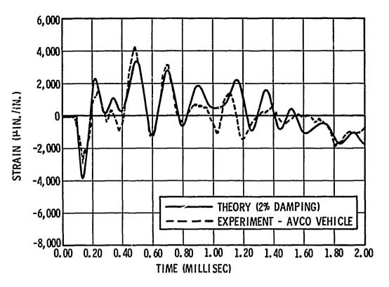
Fig. 16 - Correlation of SABOR3A/DRASTICII with Avco vehicle test data - inner fiber circumferential strain
