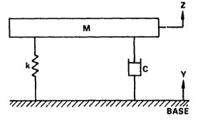
Fig. 2 - Single-degree-of-freedom mechanical system
