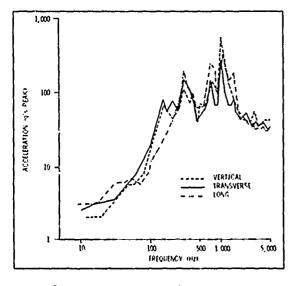
FIG. 9. Maximum Envelope of Fuze Shock Spectrum
