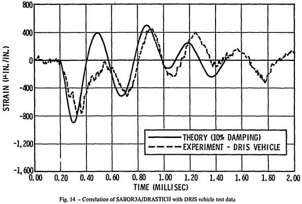
substructure circumferential strain
