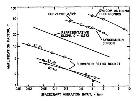
FIGURE 5. EFFECT OF STRUCTURAL DAMPING VARIATION
