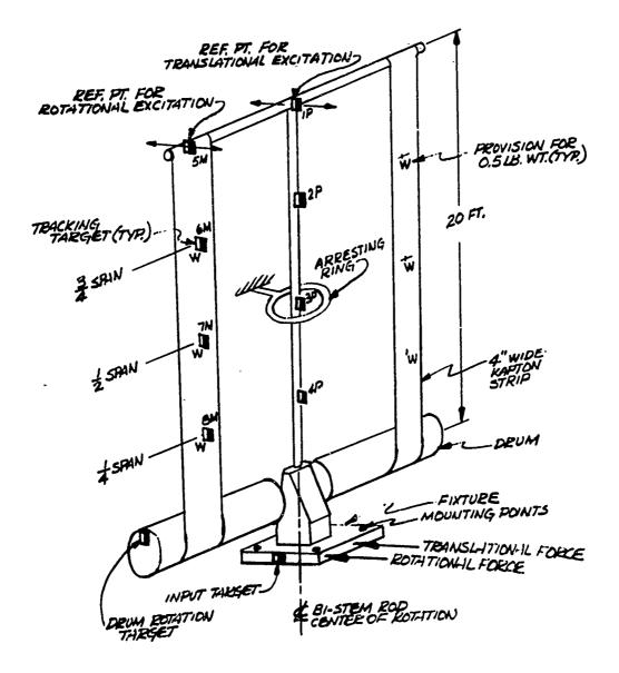
Figure 2. Phase I Test Arrangement
