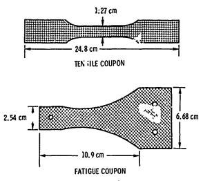
Fig. 3 - Drawings of tensile test and fatigue test models.
