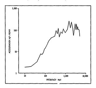
Fig. 5. Typical Undamped Shock Spectrum, (Run 1, Tail Vertical)
