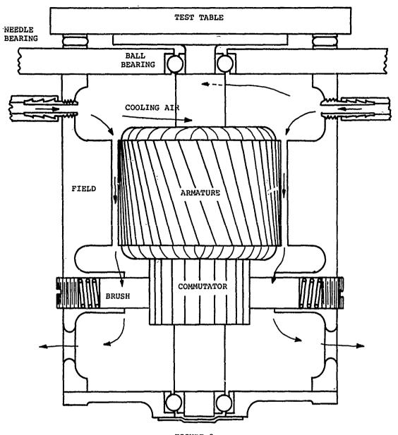
FIGURE 8 ROTATIONAL SHAKER CONSTRUCTION
