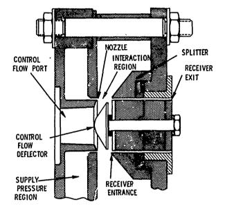
Fig. 8 - Drawing of Annular Slot model
