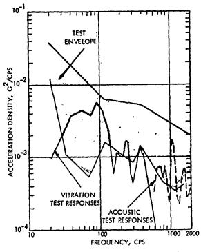
FIGURE 15 COMBINED TEST RESULTS FREE FLIGHT WARHEAD AFT MOUNT (VERTICAL)
