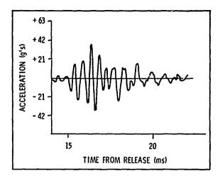
FIG. 4. Typical Acceleration Time History, (Run 1, Tail Vertical)
