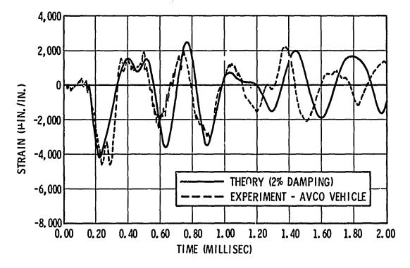
Fig. 15 - Correlation of SABOR3A/DRASTICII with Avco vehicle test data - outer fiber circumferential strain
