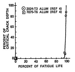
FIGURE 4. FATIGUE CRACK DEPTH GROWTH
