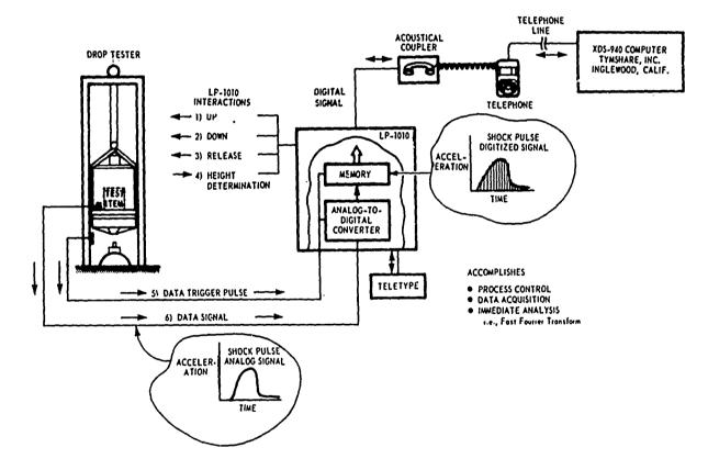
Figure 3. Drop Tester-LP-1010 Setup With Timesharing Digital Computer.
