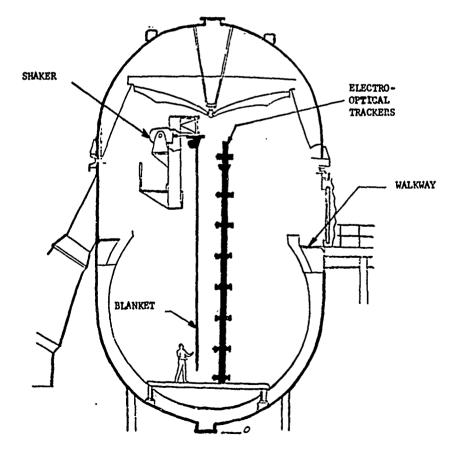
Figure 6. Deployed Modal Test Set Up
