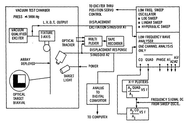
Figure 5. Block Diagram of Equipment Interrelation
