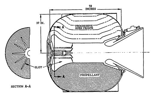
Figure 6 Cross Section of Poseidon Second Stage Motor
