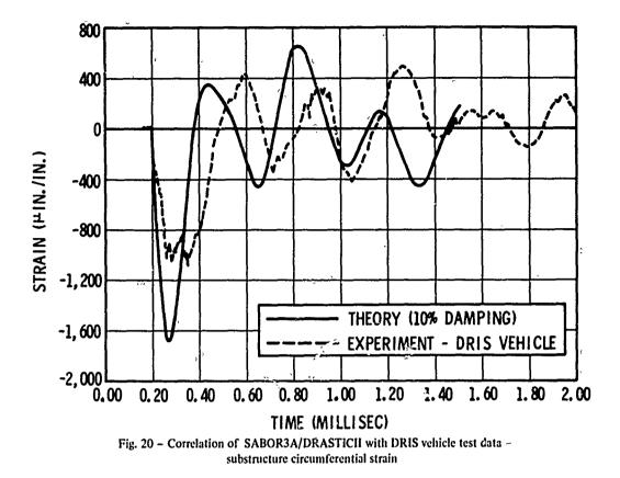
refers to SABOR3A/DRASTIC11 structural response computer code. In these strain comparison plots, the strain in microin is plotted against time in millisec. The angle designation,  $\theta$ , refers to the strain gage angle location measured from  $\theta = 0$  deg, the leading edge element line centered under the explosive load.
