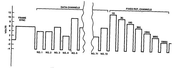
Figure 3 - Typical Scanner Output Frame
