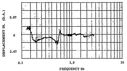
Figure 9. In-Phase Response - Translational Excitation **Ambient Pressure**
