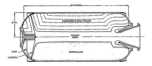
Figure 2 Cross Section of Poseidon First Stage Motor
