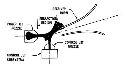
Fig. 2 - Positive Peak of an Input Cycle - Rectangular Nozzle
