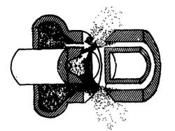
Fig. 5 - Positive Peak of an Input Cycle -Annular Slot Nozzle
