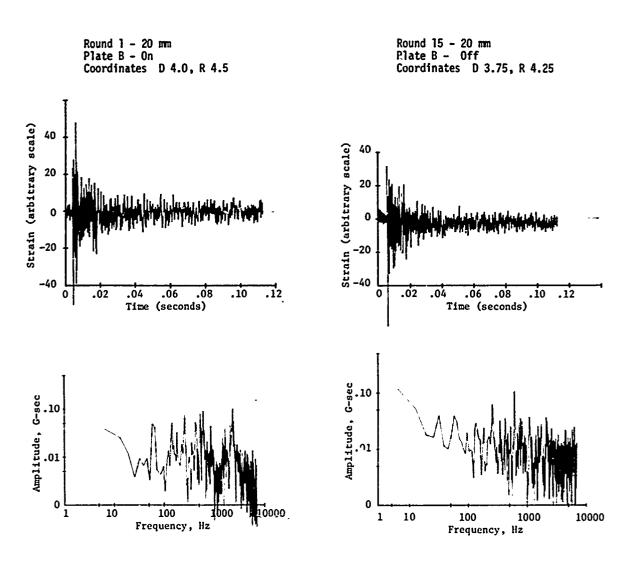
Fig. 15 - Strain gage traces and Fourier amplitude
