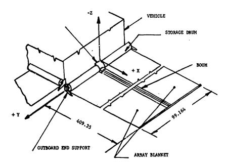
Figure 1. Roll-Up Solar Array Configuration (Coordinate System Shown)
