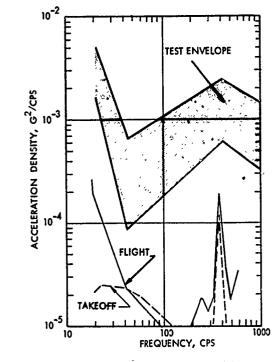
FIGURE 11 DERIVED TEST ENVELOPES ELECTRONICS SECTION CASTING(FORE/AFT) (U) Initial vibration input equalization iterations were performed on a dummy missile to minimize environmental.exposure of the qualification hardware and to acquire confidence in the test procedure.
