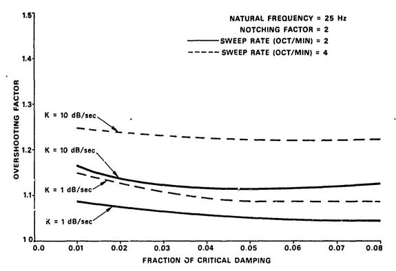
Fig. 6 - Overshooting factor for automatic notch control system
