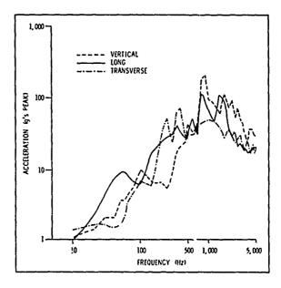
FIG. 10. Maximum Envelope of Guidance Shock Spectrum
