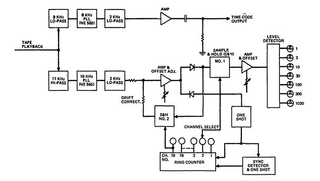
Figure 2 - Decoder Block Diagram
