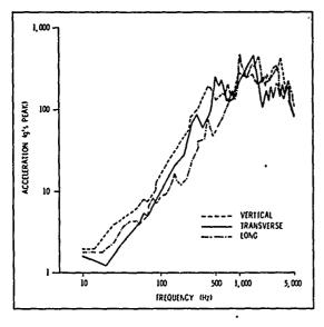
FIG. 8. Maximum Envelope of Tail Shock Spectrum
