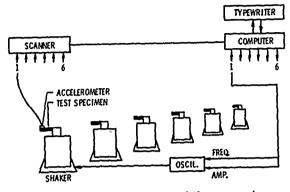
Fig. 6 - Schematic diagram of the computer control for fatigue testing of acoustic materials.
