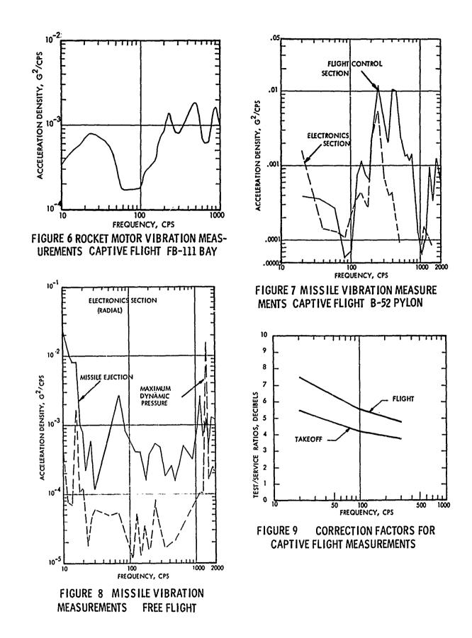
Flight measured data for these test segments were increased by scaling the dynamic pressure to maximum design conditions. The corrections include a factor equivalent to a 4X increase in the design service exposures, which is consistent with the required fatigue design practice. The resulting test durations were 8 hours for captive flight, 5 minutes for weapon bay buffet and 8 minutes for free flight.
