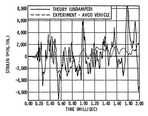
Fig. 17 Correlation of SABOR3A/DRASTICH undamped analysis with Avco vehicle test data - outer fiber meriodional strain
