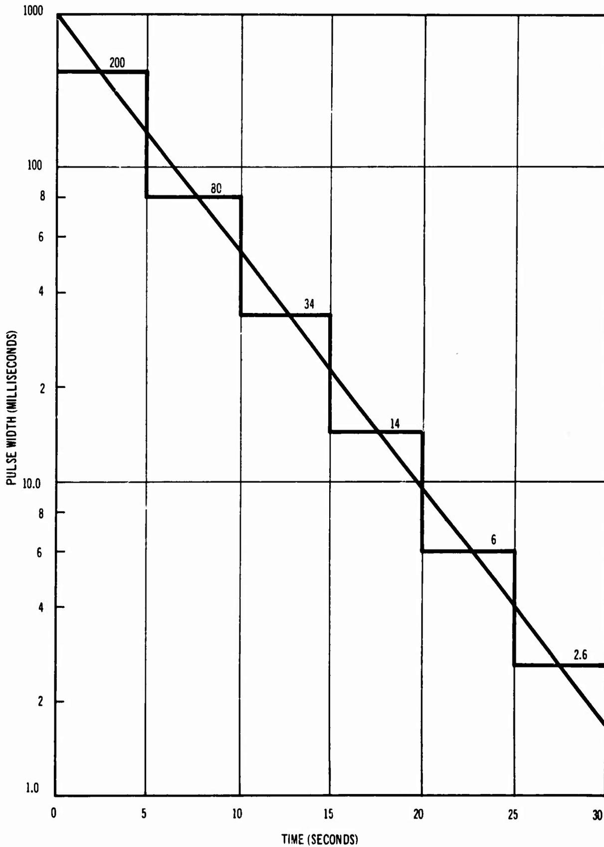
Figure C-1. Pulse Width vs Time of Output Stage
