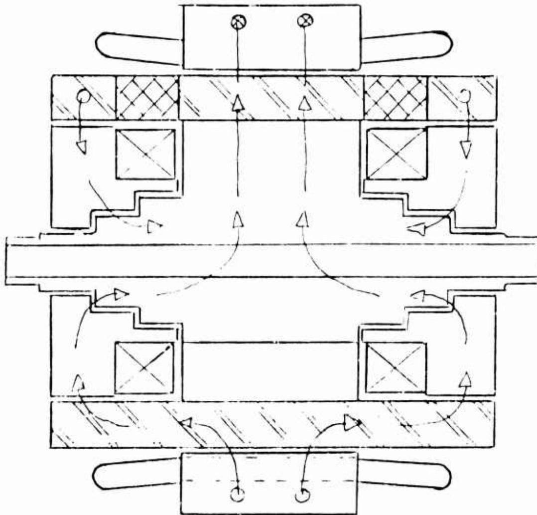
A brushless, stationary-coil Lundell-type generator that uses two exciting coils is described in U. S. Patent 2,796,542 issued to A. Becky.
