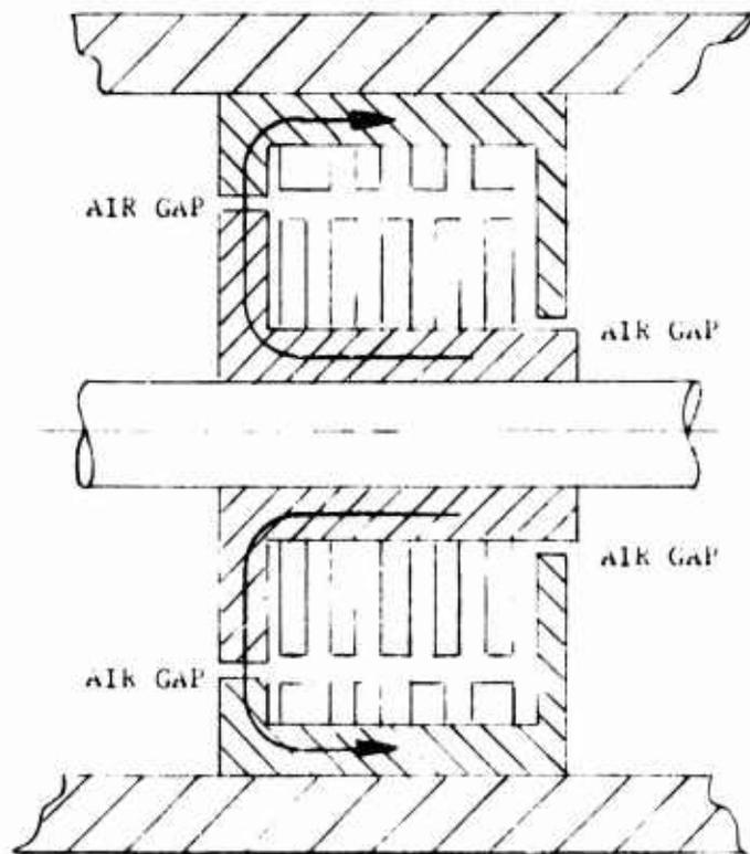
MAGNETIC FLUX PATTERN OF ROTARY TRANSFORMER
