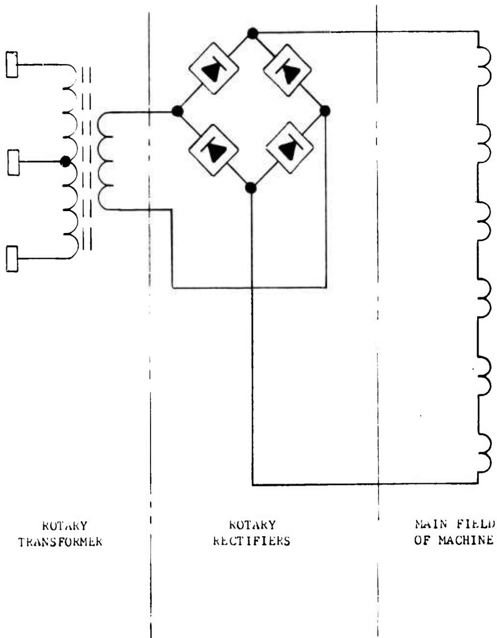
ROTARY TRANSFORMER-RECTIFIER ASSEMBLY
