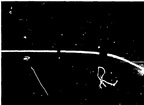
50 keV electrons interacting with nitrogen at 80 millitorr produce an intense luminescent beam. The center of the beam is N 2 + emission produced by primary electrons. The diffuse emission outside the primary beam is due to N 2 excited by low energy secondary electrons.
