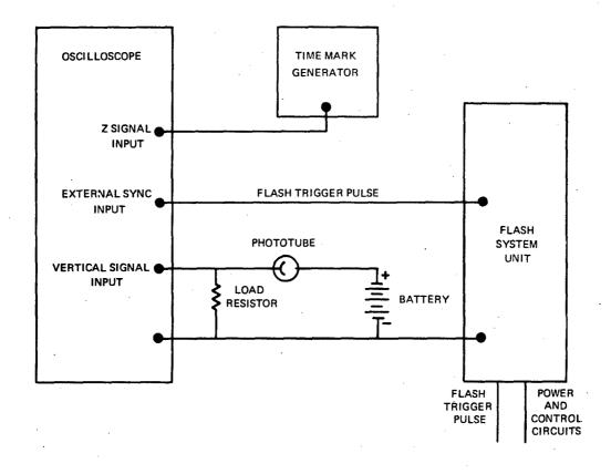
Figure 1. Type Equipment Arrangement for Test of Flash Duration and Flash Repetition Rate.
