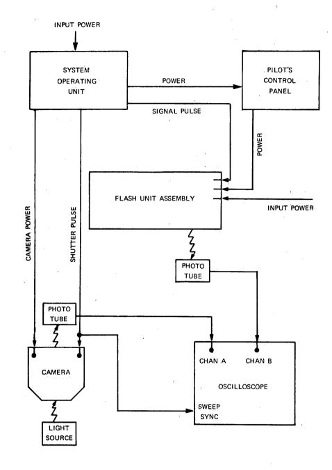
Figure 2. Type Equipment Arrangement for Synchronous Operation Test.
