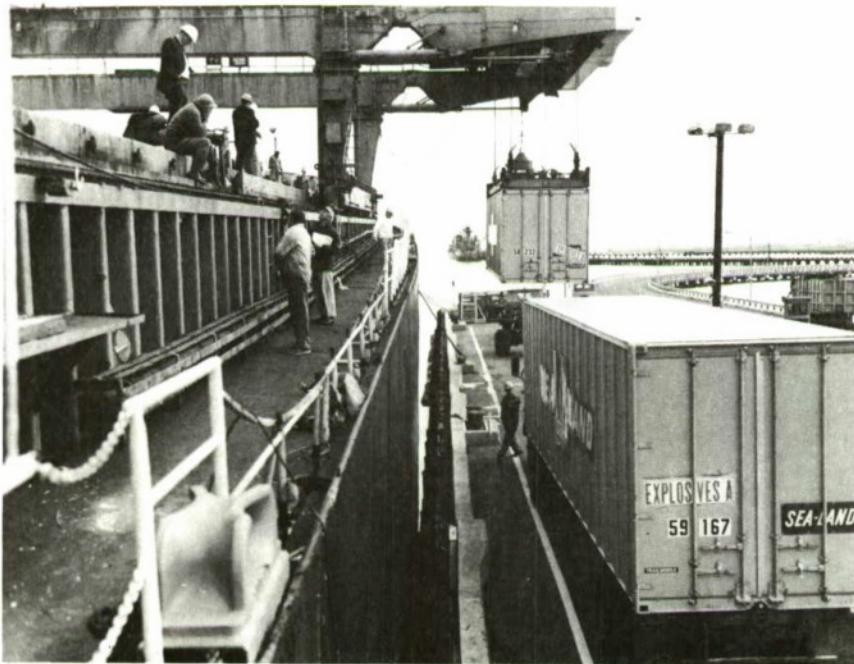
Figure 18. Container Being Lifted Aboard; Note White Guide Line on Pier to Assist Drivers in Positioning Containers.
