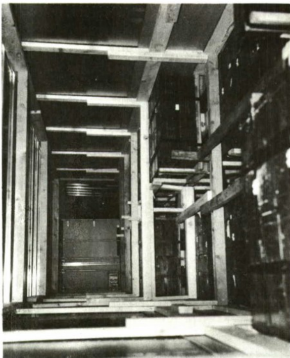
Figure 9. Container Number 59241, Front to Rear View of Small Arms Ammunition Showing Blocking and Bracing in Need of Tightening.
