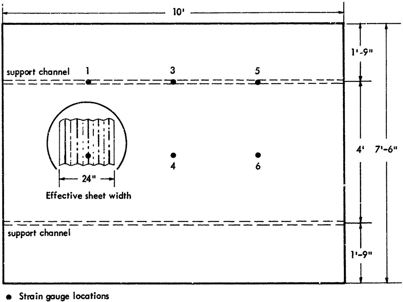
Fig. 3. Corrugated Steel Test Wall
