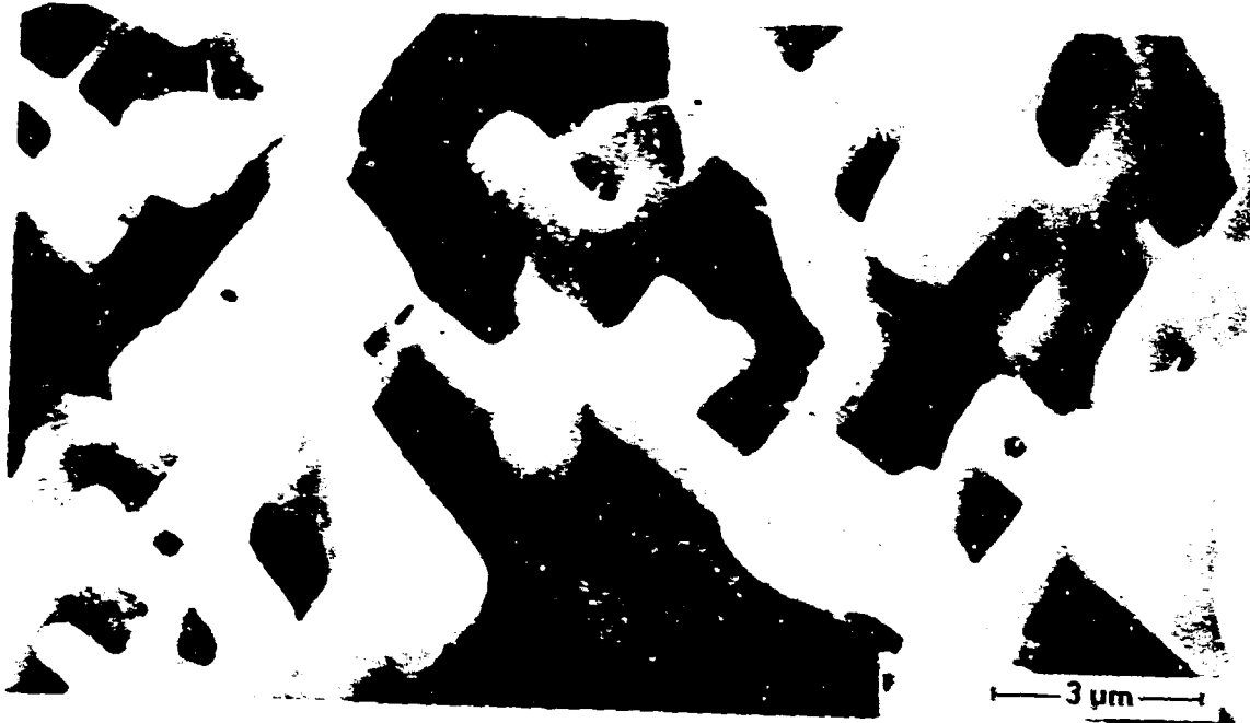
Low temperature decomposition at 230°C for 500h
