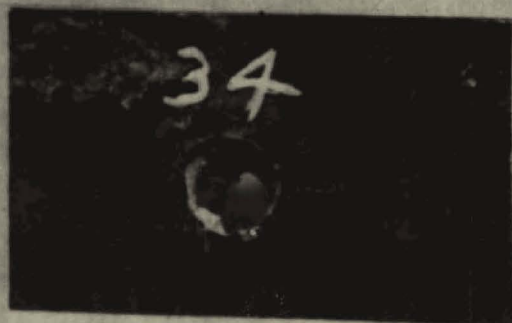
Fig.3 Grade: Standard Plate Round Velocity Normal Impact 5 34 2832 Penetration Navy Complete
