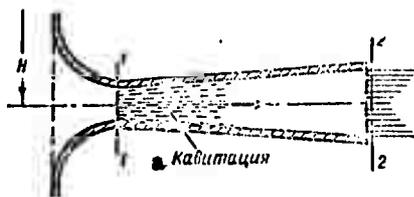
Fig. 98. Diffuser mouthpiece.
