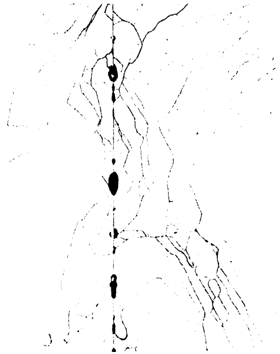
Photomicrographs of a niobium bicrystal boundary, showing decrease in porosity and accompanying dislocation density. Top: As welded. Bottom: Electroetched to develop pits at dislocation sites. Magnification: 100X.
