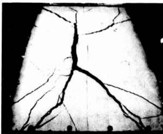
e. 1512 psf ( 7382.2 \text{ kg/m}^2 ), failure
