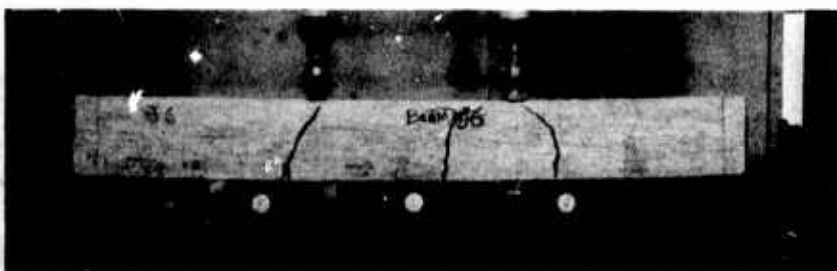
d. Total load = 3800 lb (1723.6 kg), failure
