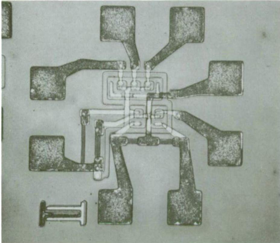
Figure 21. Photomicrograph of 1 mW, high speed ECL gate (SMX8).
