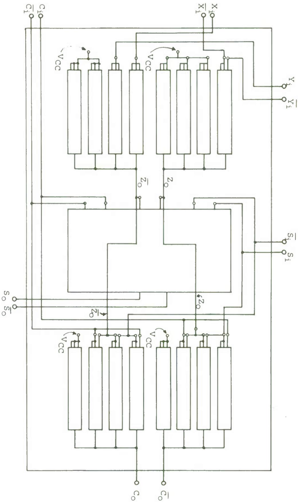
Note: This diagram illustrates the implementation of the circuitry of three 3-Bit Parity Cells to form the Multiplier. The small rectangles represent the basic 3-input gates of the parity cell; the large rectangle represents a 3-Bit Parity Circuit.
