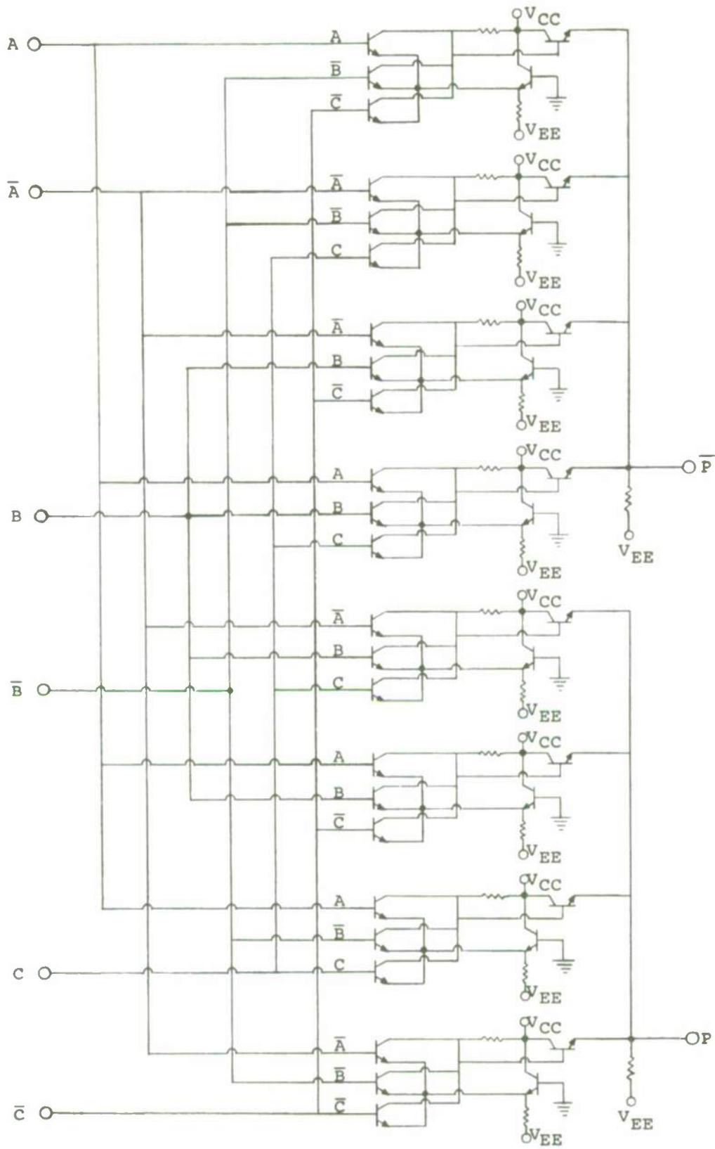
Figure 5. Schematic diagram of 3-Bit Parity Array.
