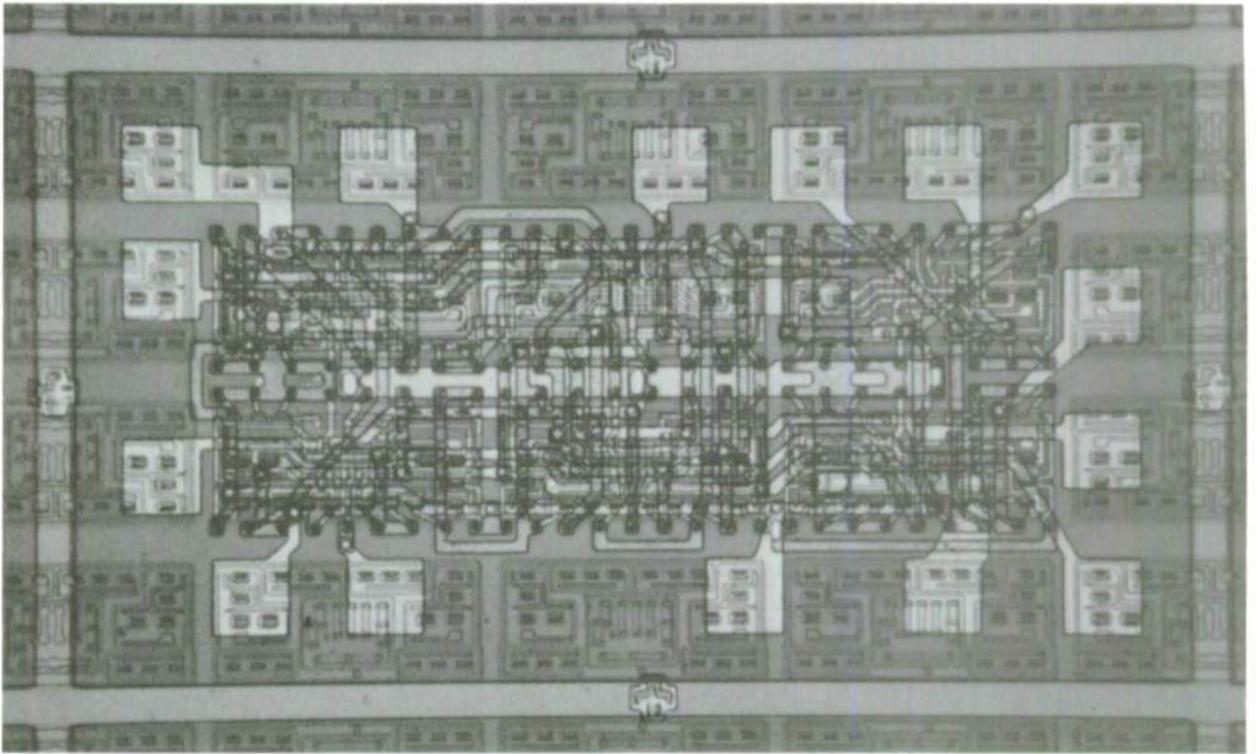
Figure 12. 1 x 1 Functional Multiplier Array.
