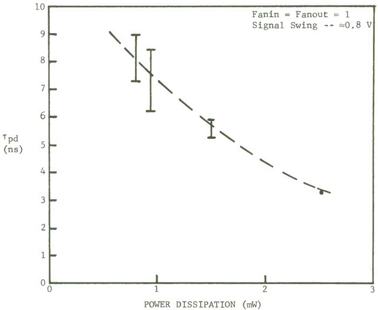
Figure 22. Propagation delay time versus power dissipation for the emitter follower input, complementary output, ultrasmall geometry ECL gate (SMX8).
