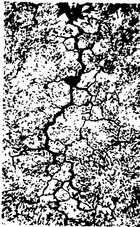
Fig. 31 Deep intergranular microcrack (18% Ni, 200 ksi*) exposed as two-point-loaded specimen at 200 ksi for 247 days in 80 ft lot at Kuré Beach. Etchant: modified Fry's reagent
