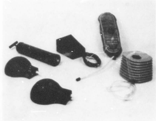
Figure 10 - Commercial Foot Pumps Evaluated
