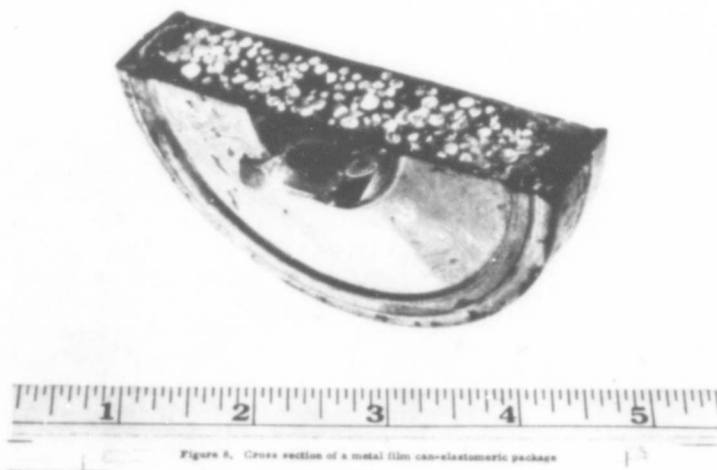
Figure 8. Cross section of a metal film can-elastomeric package
