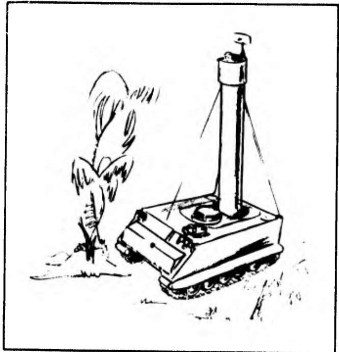
Figure 26 - Observation Tower Mounted in M-106
