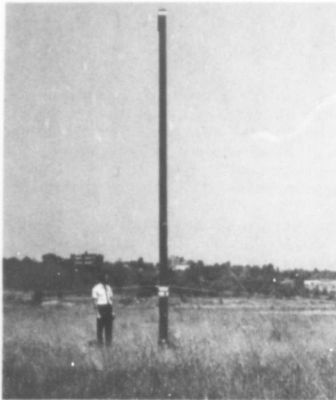
Figure 1 (Above) - Sixty-Foot VHF-UHF Manpack Antenna Mast; Figure 2 (Below) - Top-Loaded LF Antenna Mast
