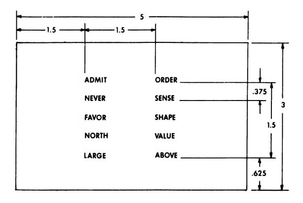
Fig. 1. ARRANGEMENT AND DIMENSIONS (INCHES) OF TEST CARDS
