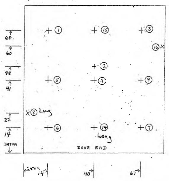
Notes: Thermocouples #16 and # 8 to be attached to inner skin on side walls as shown 40 inches from floor.
