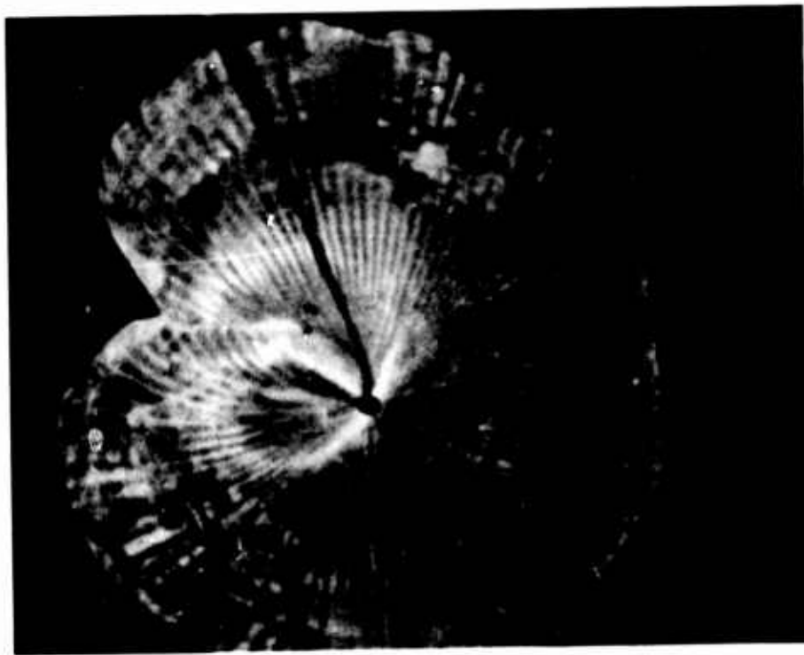
Figure 15. Top View of Flight No. 3 at 57,250 Ft, Clearly Showing the Effects of the Increasing Forces of Deployment on the Undeveloped Pocket Corners and Circumferential Stress Band
