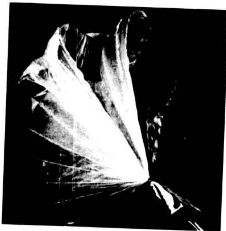
Figure 17. Up-Camera View of Flight No. 3 at 65,000 Ft, 2 to 3 Sec Before Burst, Showing the Back Side of the Subpressure Cavity During Sailing
