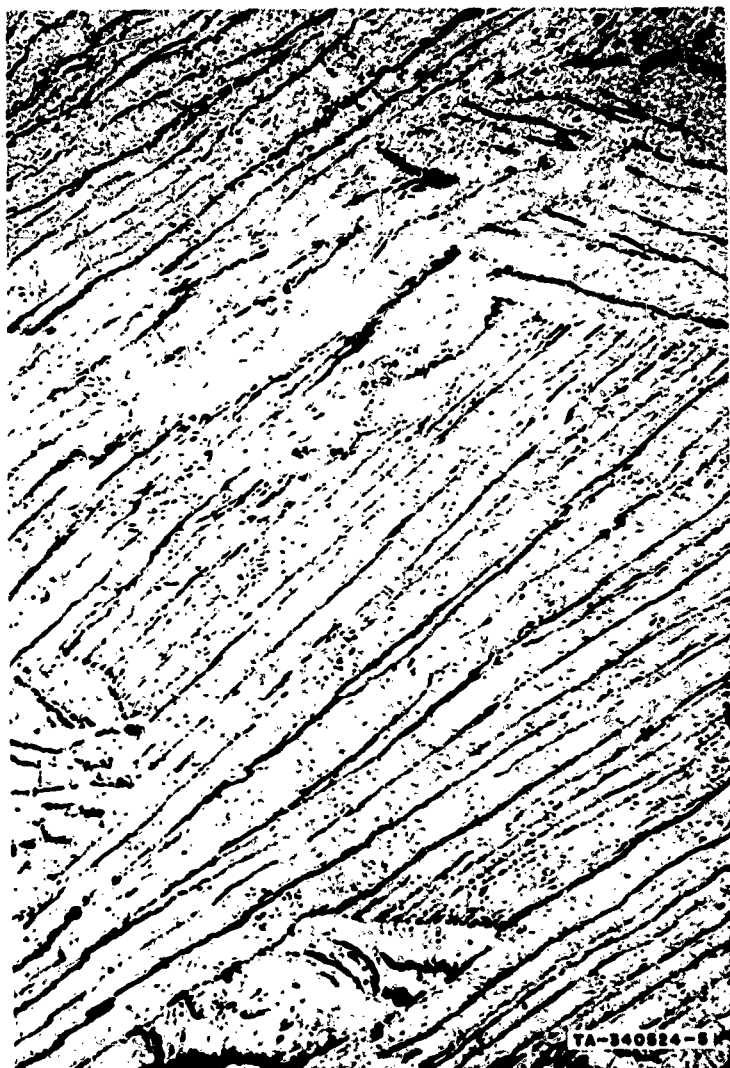
FIG. 3 LIGHT MICROGRAPH OF 70% COLD ROLLED Ti-3 wt % Cu TITANIUM 200X (4 × 5 in. enlarged to 5 × 7 in.). Etchant 25 ml HNO 3 , 25 ml H 2 O, 1 ml HF.
