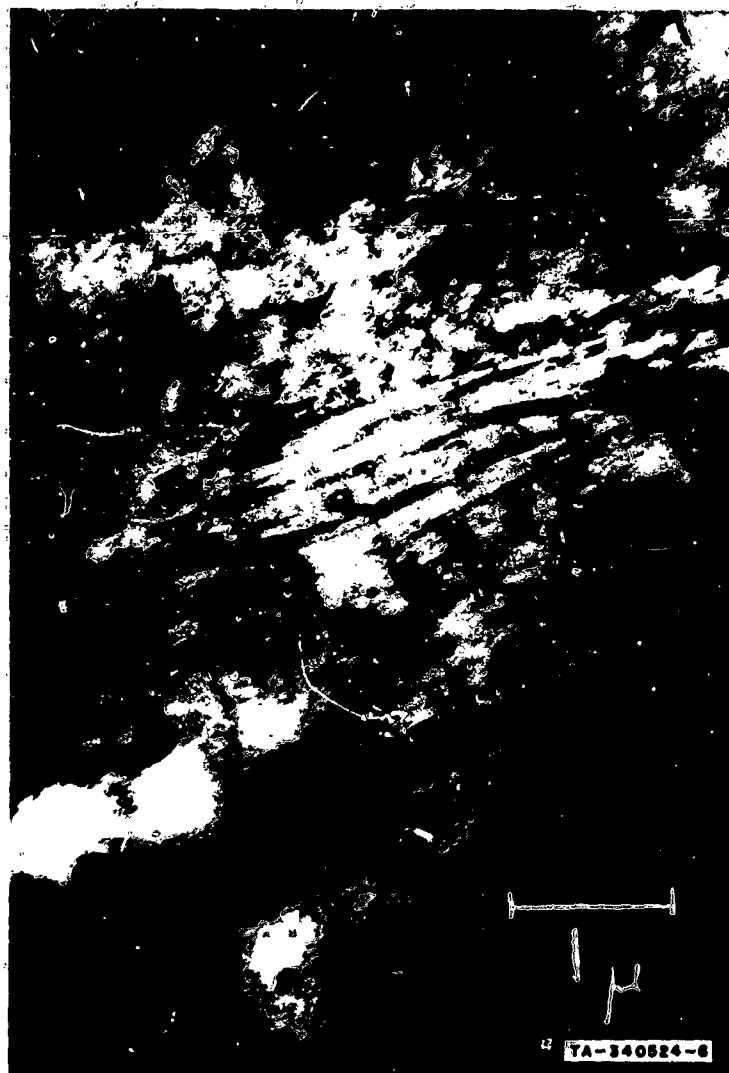
FIG. 4 TRANSMISSION ELECTRON MICROGRAPH, 25,000X Pearlite-like eutectoid structure becomes elongated and width reduced. \alpha : \text{Ti}_2\text{Cu} width ratio is about 2:1. Cell structure forming in area free of lamellar structure. Cell size \sim 0.4\mu .
