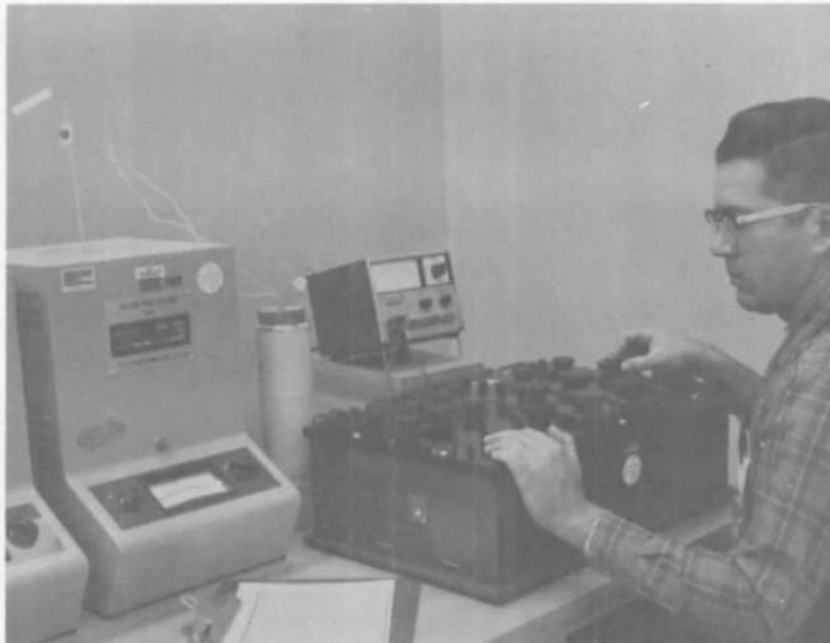
The Output of a Thermocouple is Measured at the Freezing Point of a Pure Metal.
