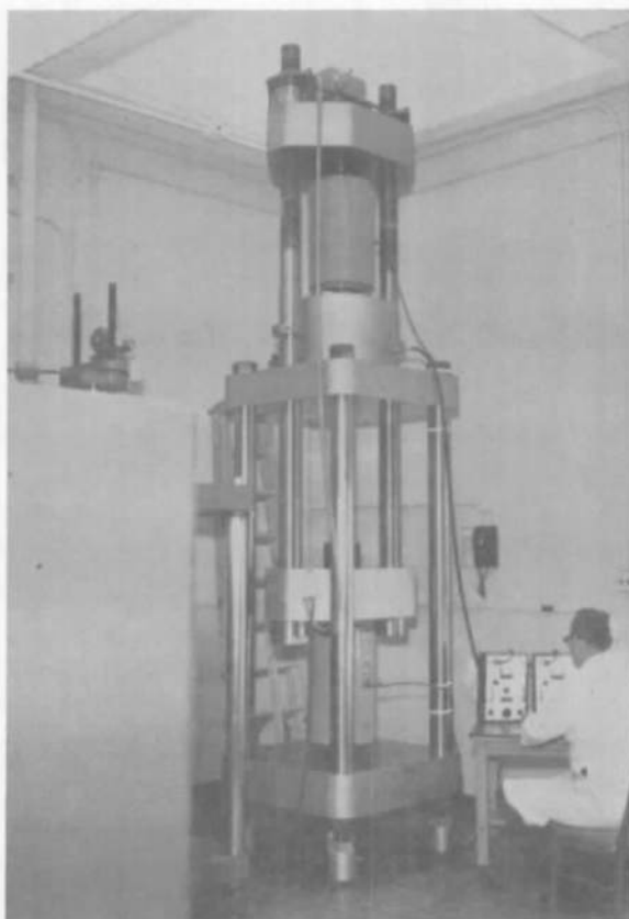
Two 500,000-lb Load Cells are Compared Using an Hydraulic Calibrator.
