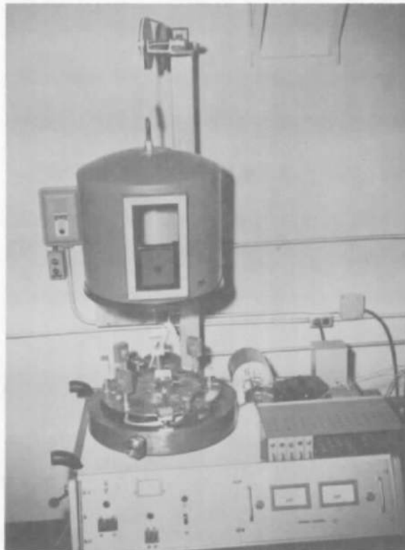
Equipment Used for the Calibration of Total Radiation Detectors under Vacuum
