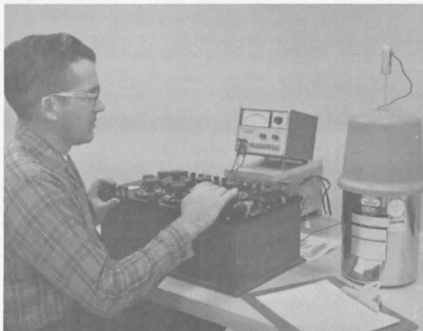
A Resistance Thermometer is Checked at the Triple Point of Water.
