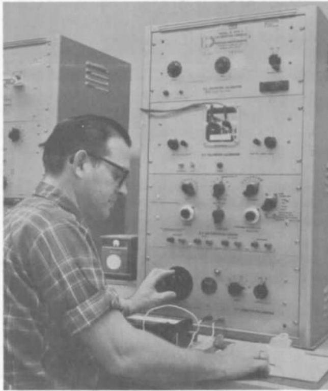
Rapid Calibration of Electrical Indicating Meters is Possible Using Specialized Equipment.
