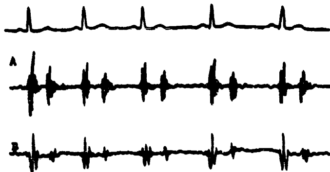
Fig. 67. Seismocardiograms recorded by "EMA" plant pickups (A) and N. G. Esaulov's pickup (B). Electrocardiogram at top.
