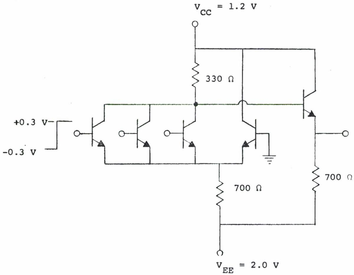
Figure 2. Basic 3-input gate for parity array.
