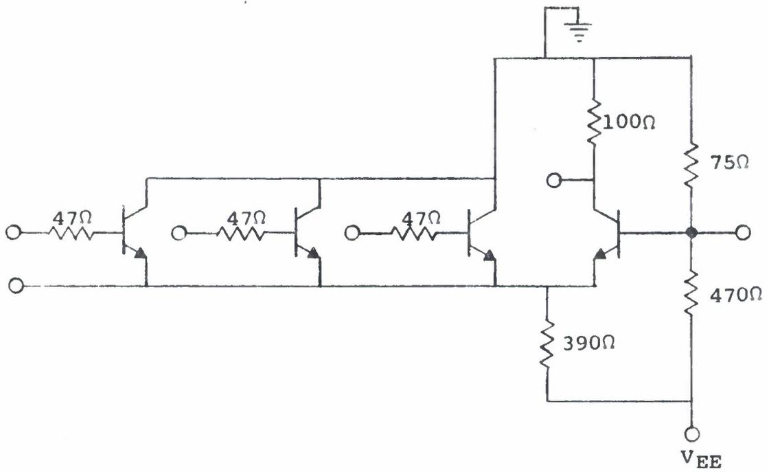
Figure 4. SMX3, Microcircuit Version of ECL Type Circuit.
