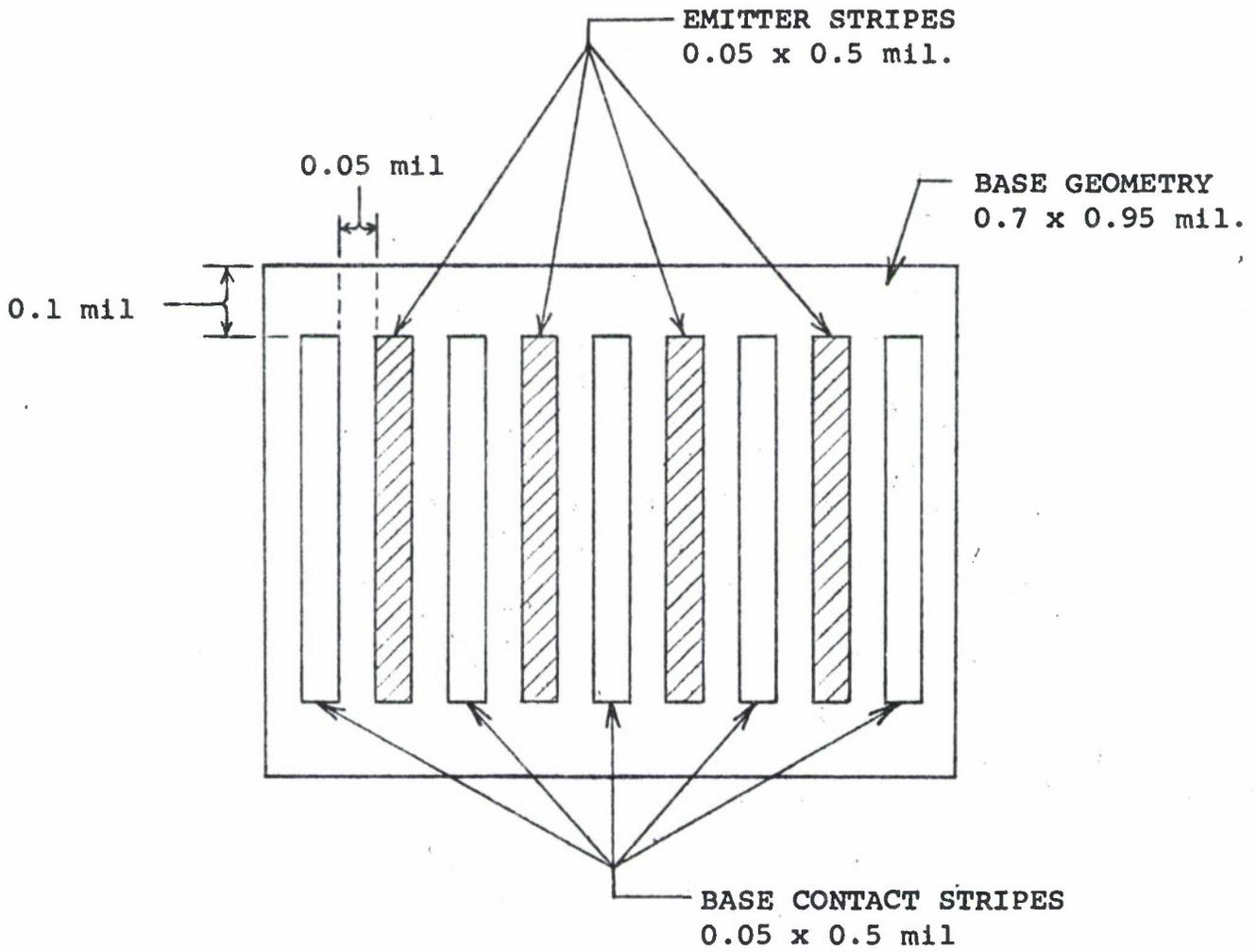
Figure 1. SX4 transistor geometry.
