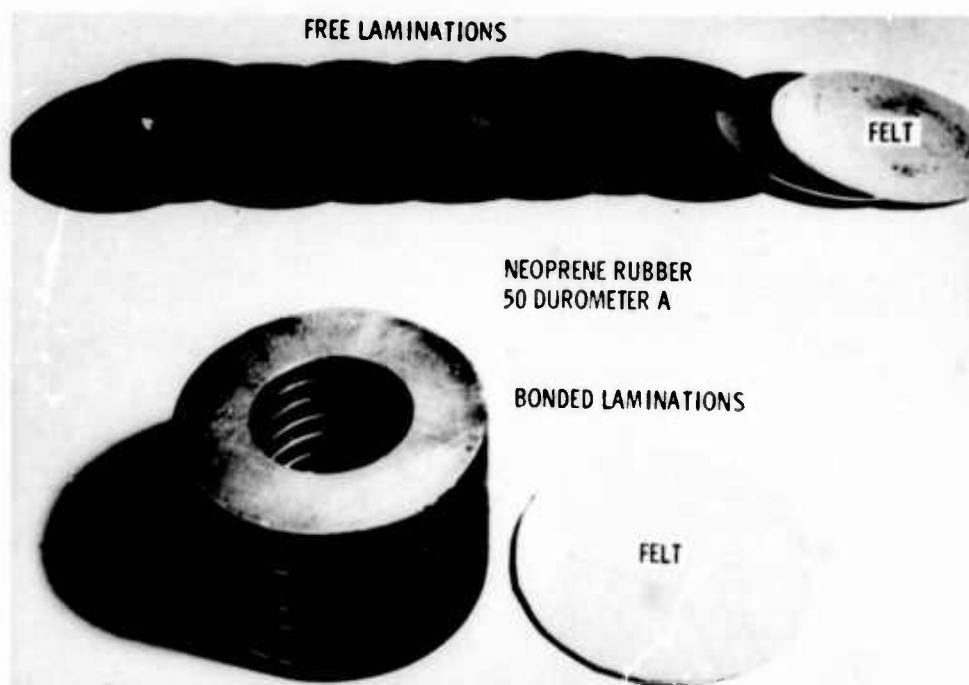
Fig. 5. Rubber spring having different boundary conditions
