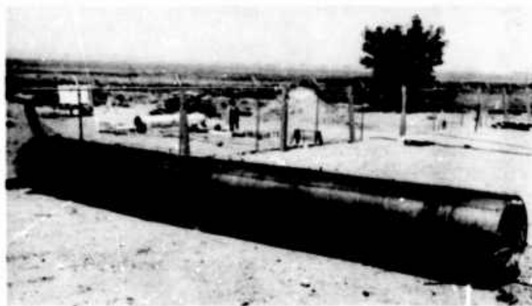
Fig. 11. Perforated metal liner and explosive strand array for 130-ft gun test
