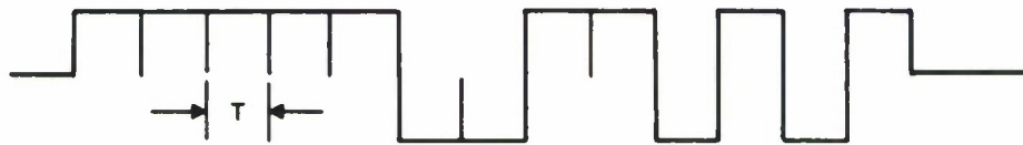
(b) THE WAVEFORM AT THE OUTPUT OF THE FILTER OF FIG. 73 (TERMINAL 2)
