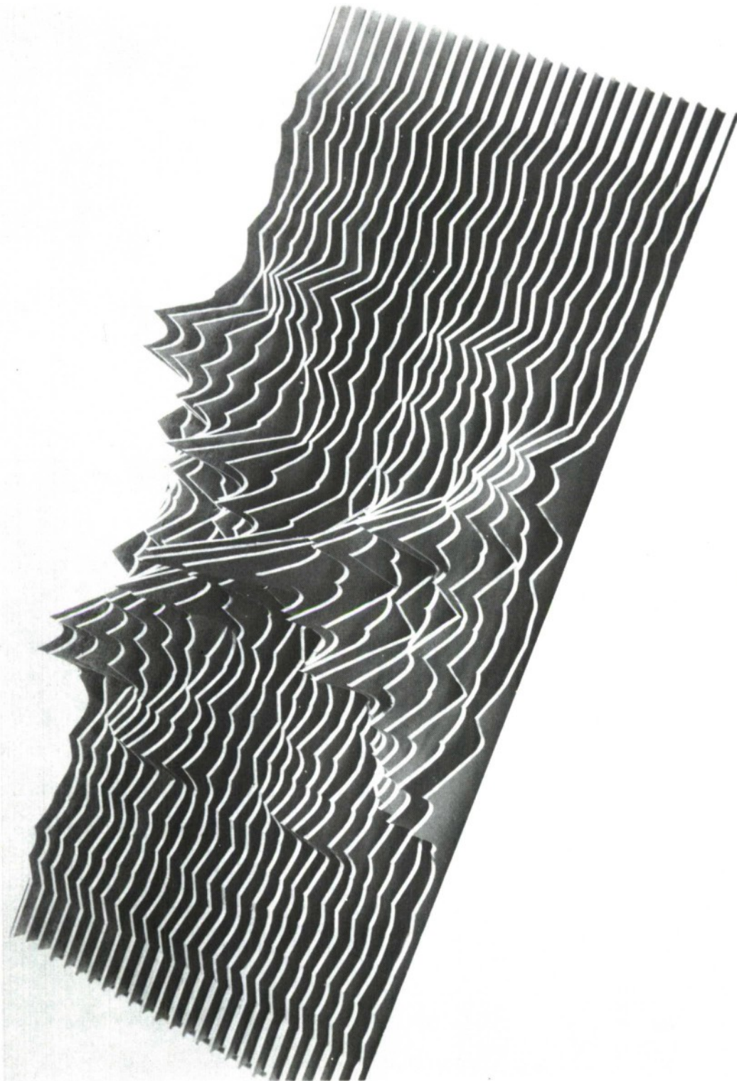
Fig. 36 The two-dimensional correlation function of the 13-code signal. Profiles are taken vs. time at intervals of 1/4 \Delta in Doppler, where \Delta is the duration of the signal. (Taken from Key et al., Ref. 31, with permission.)
