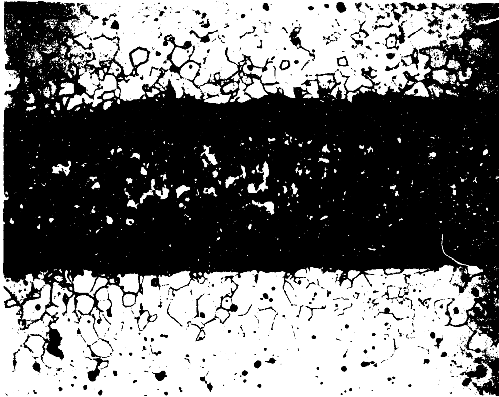
Figure 28 - Photomicrograph of seal sample 1-5B, transverse section, after 144 hours at 900 o C in 100 Torr of cesium vapor, 100 X
