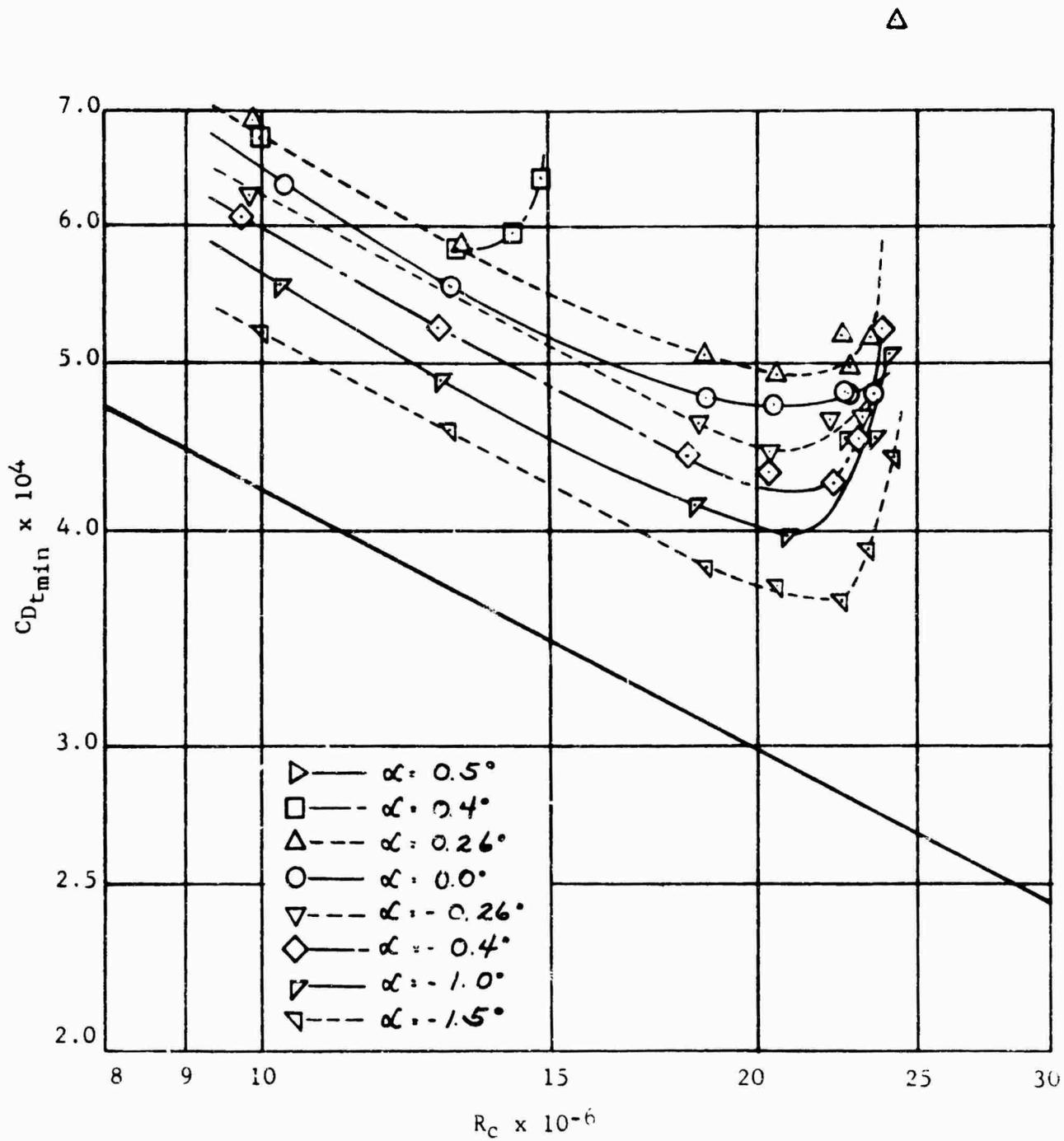
FIGURE 47 VARIATION OF MINIMUM TOTAL DRAG COEFFICIENT  $C_{Dt}$
