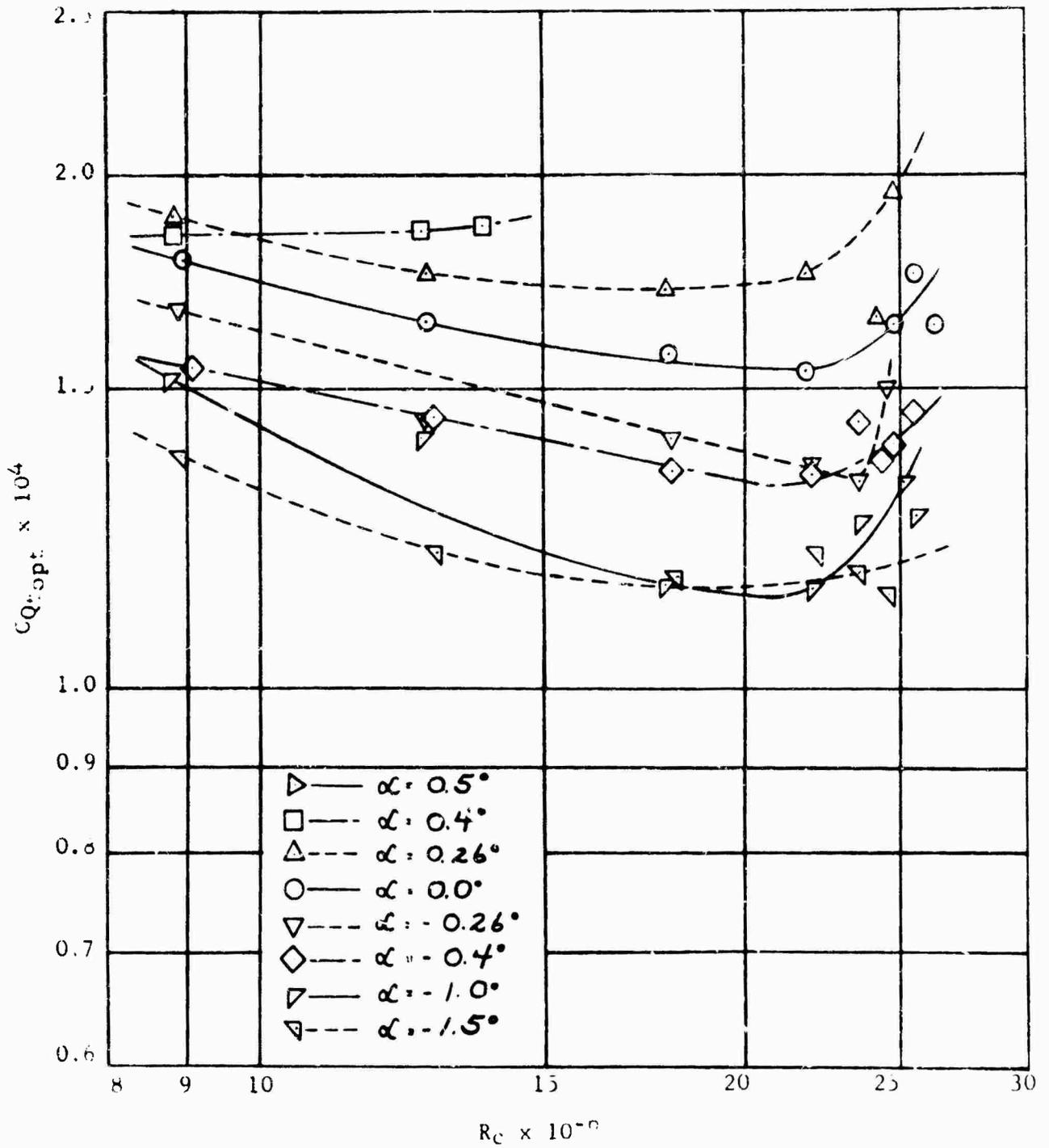
FIGURE 46 VARIATION OF OPTIMUM SUCTION COEFFICIENT  $C_{Qt_{opt}}$  WITH REYNOLDS NUMBER  $R_c$  FOR SEVERAL ANGLES OF ATTACK  $\alpha$
