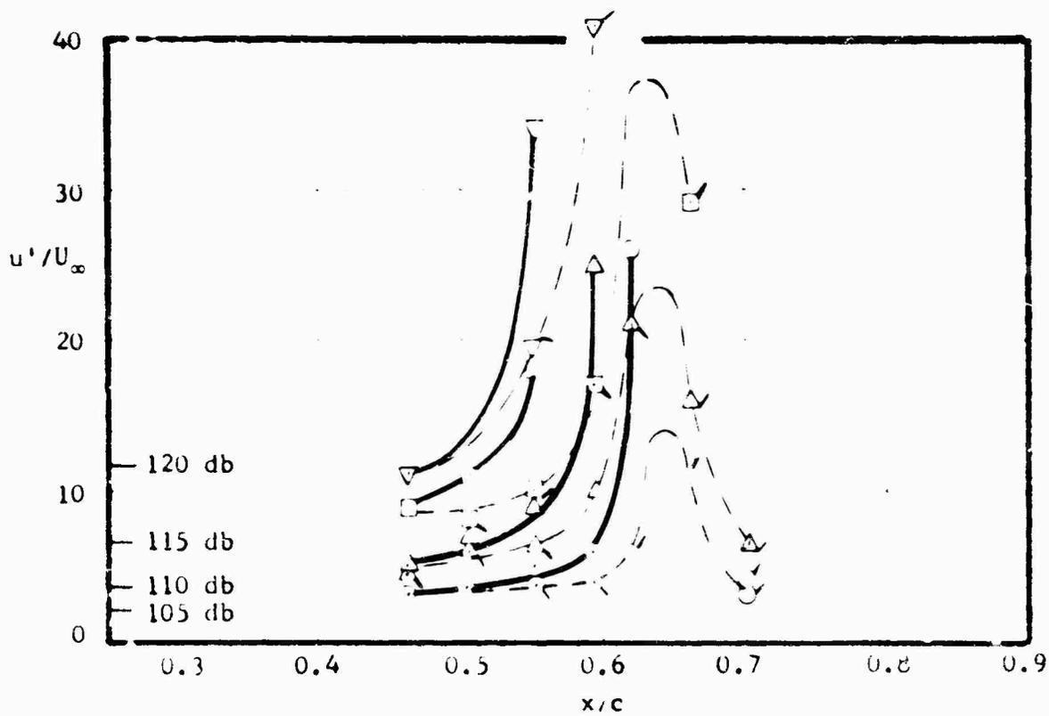
FIGURE 13. BOUNDARY LAYER FLUCTUATIONS AT VARIOUS CHORD LOCATIONS,
