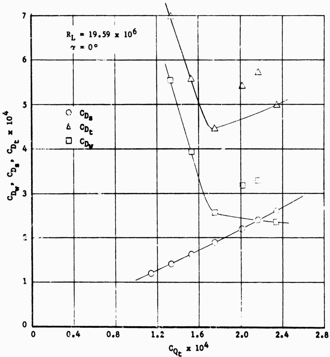
FIGURE 173 DRAG  $C_D$  VERSUS SUCTION QUANTITY  $C_{Qt}$  FOR VARIOUS REYNOLDS NUMBERS  $R_c$  AND ANGLES OF ATTACK  $\alpha$
