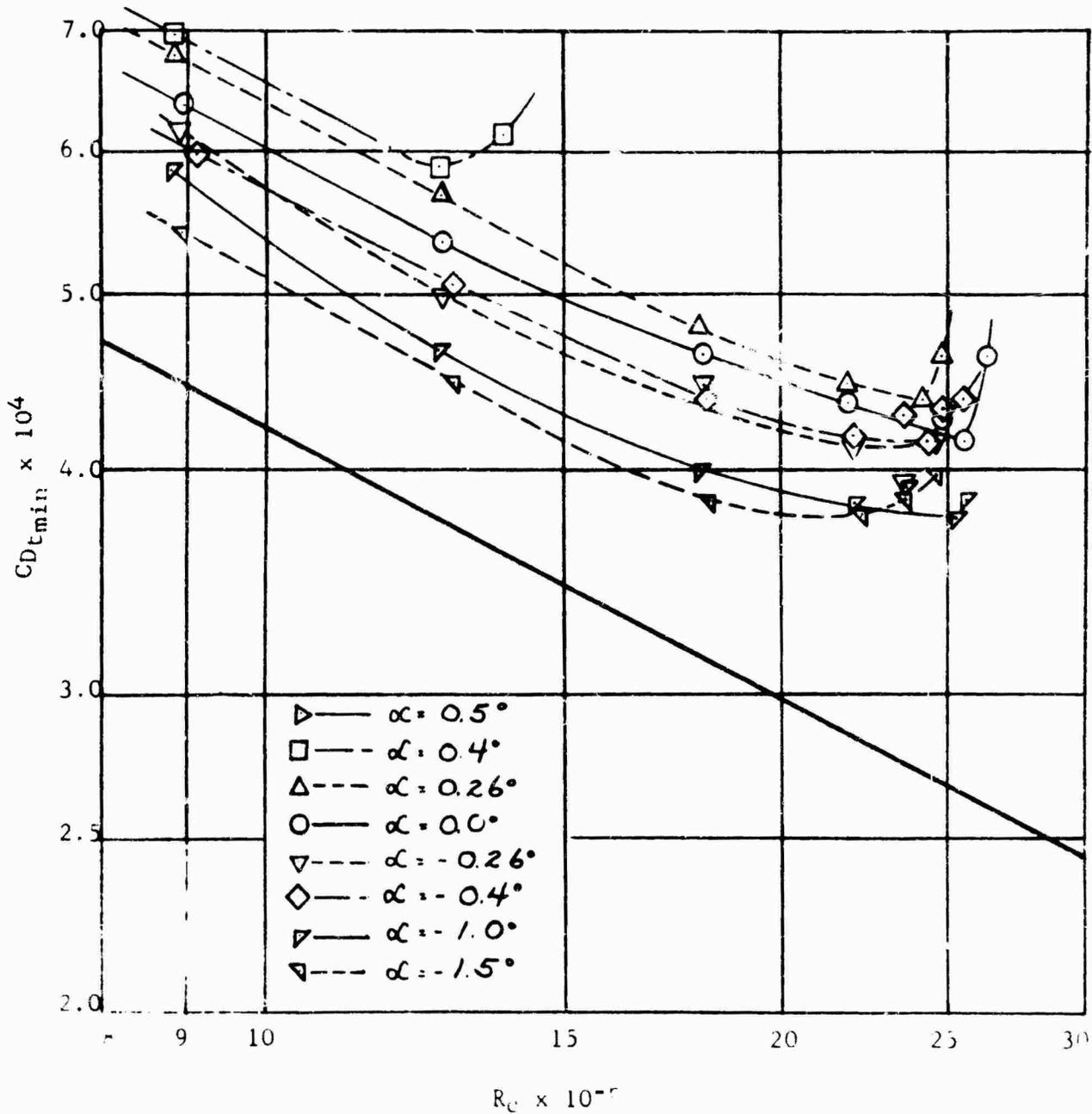
FIGURE 45 VARIATION OF MINIMUM TOTAL DRAG COEFFICIENT  $CD_t$  (INCLUDING EQUIVALENT SUCTION DRAG) WITH REYNOLDS NUMBER  $Re$  FOR SEVERAL ANGLES OF ATTACK  $\alpha$
