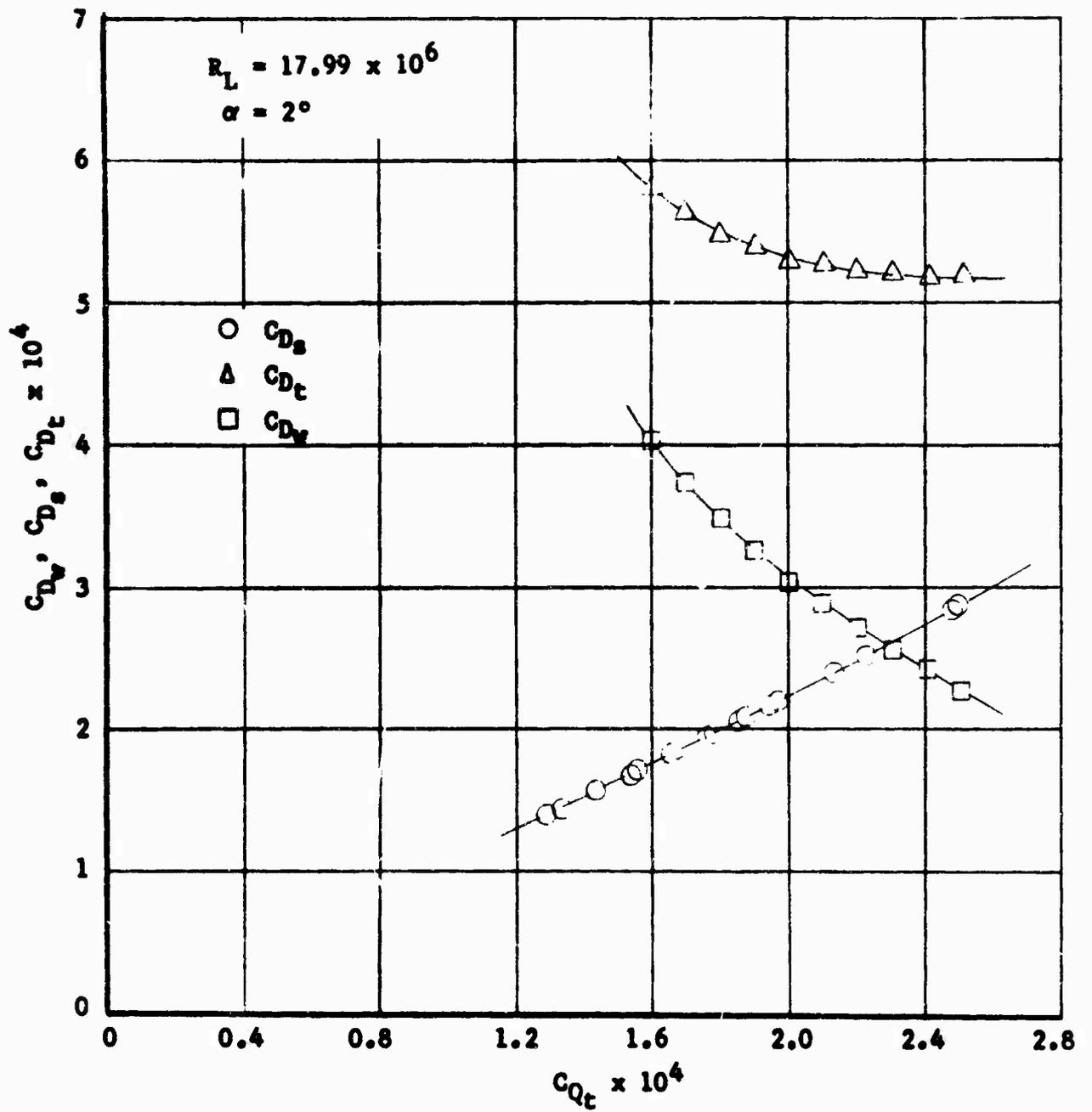
FIGURE 182 DRAG  $C_D$  VERSUS SUCTION QUANTITY  $C_{Q_c}$  FOR VARIOUS REYNOLDS NUMBERS  $R_c$  AND ANGLES OF ATTACK  $\alpha$
