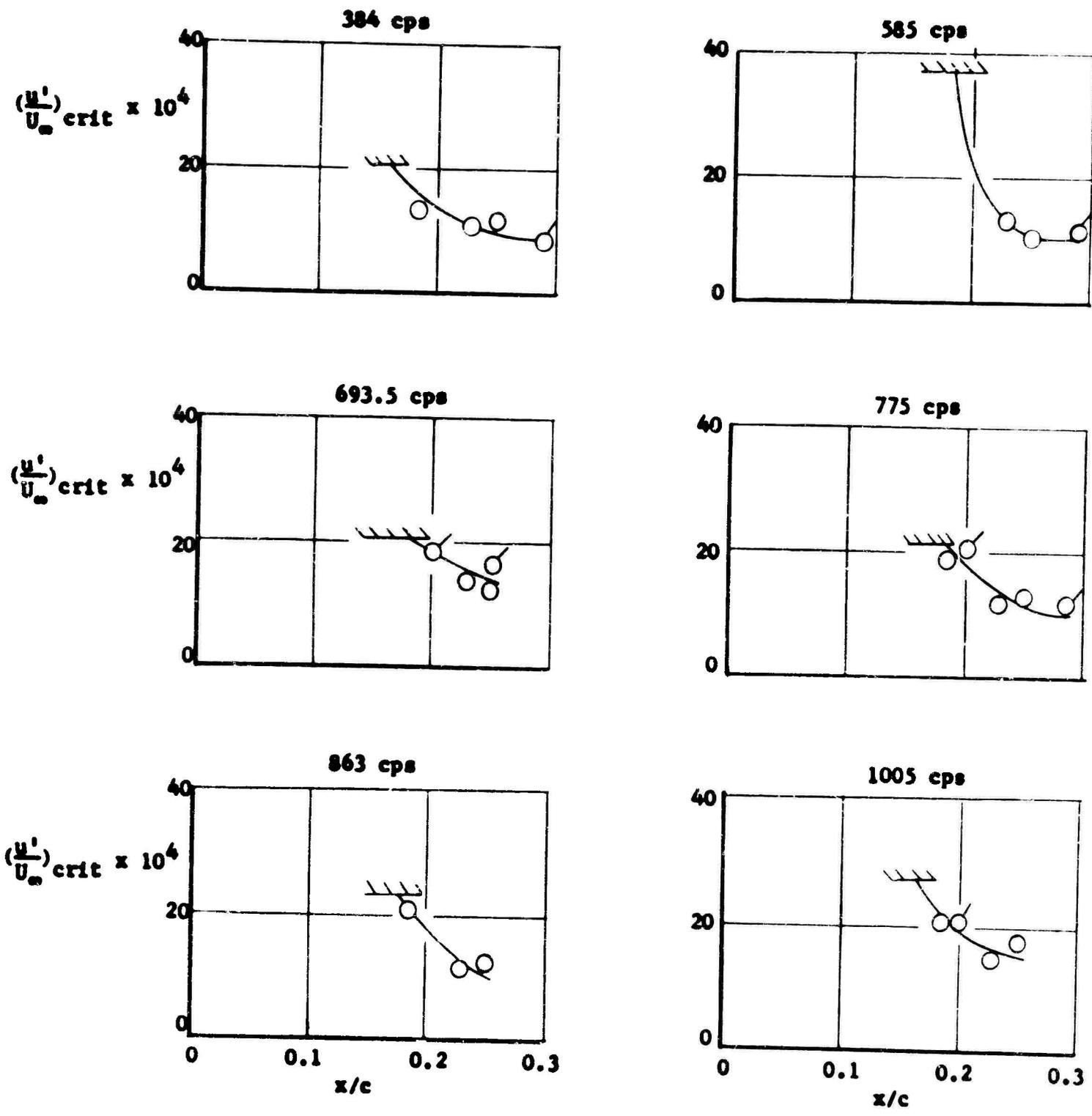
FIGURE 136 EXTERNAL SOUND LEVEL TO CAUSE TRANSITION AS A FUNCTION OF CHORDWISE LOCATION OF TRANSITION,  $R_c = 14.2 \times 10^6$
