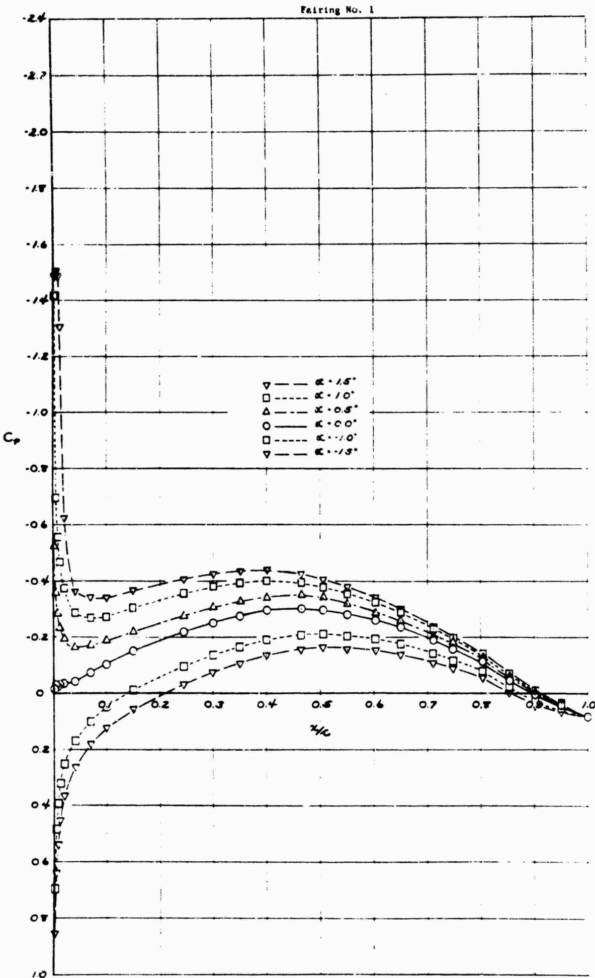
FIGURE 3.5 PRESSURE DISTRIBUTIONS AT VARYING ANGLES OF ATTACK
