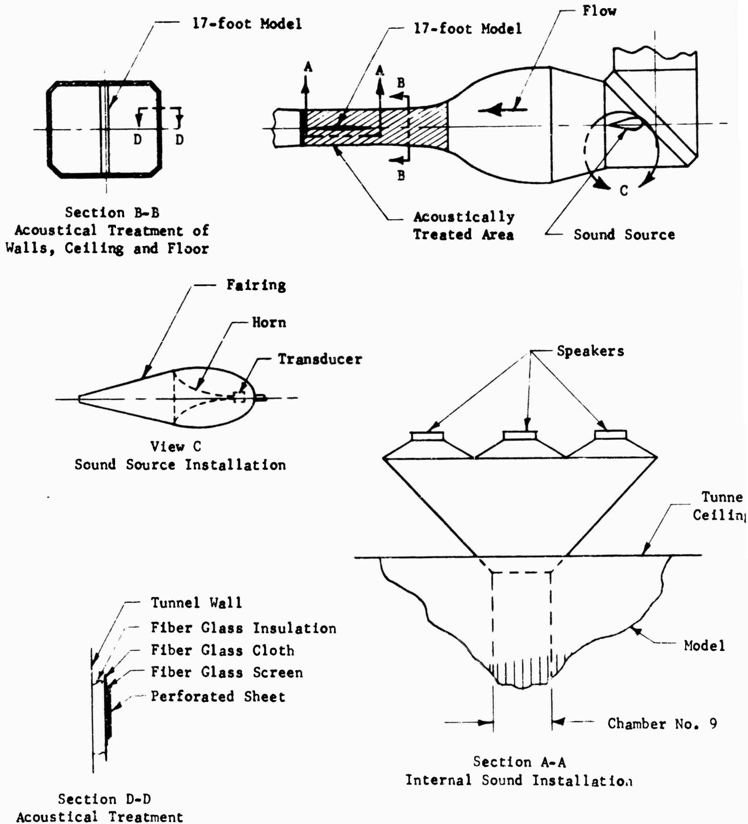
FIGURE 66 ACOUSTICAL INSTALLATION
