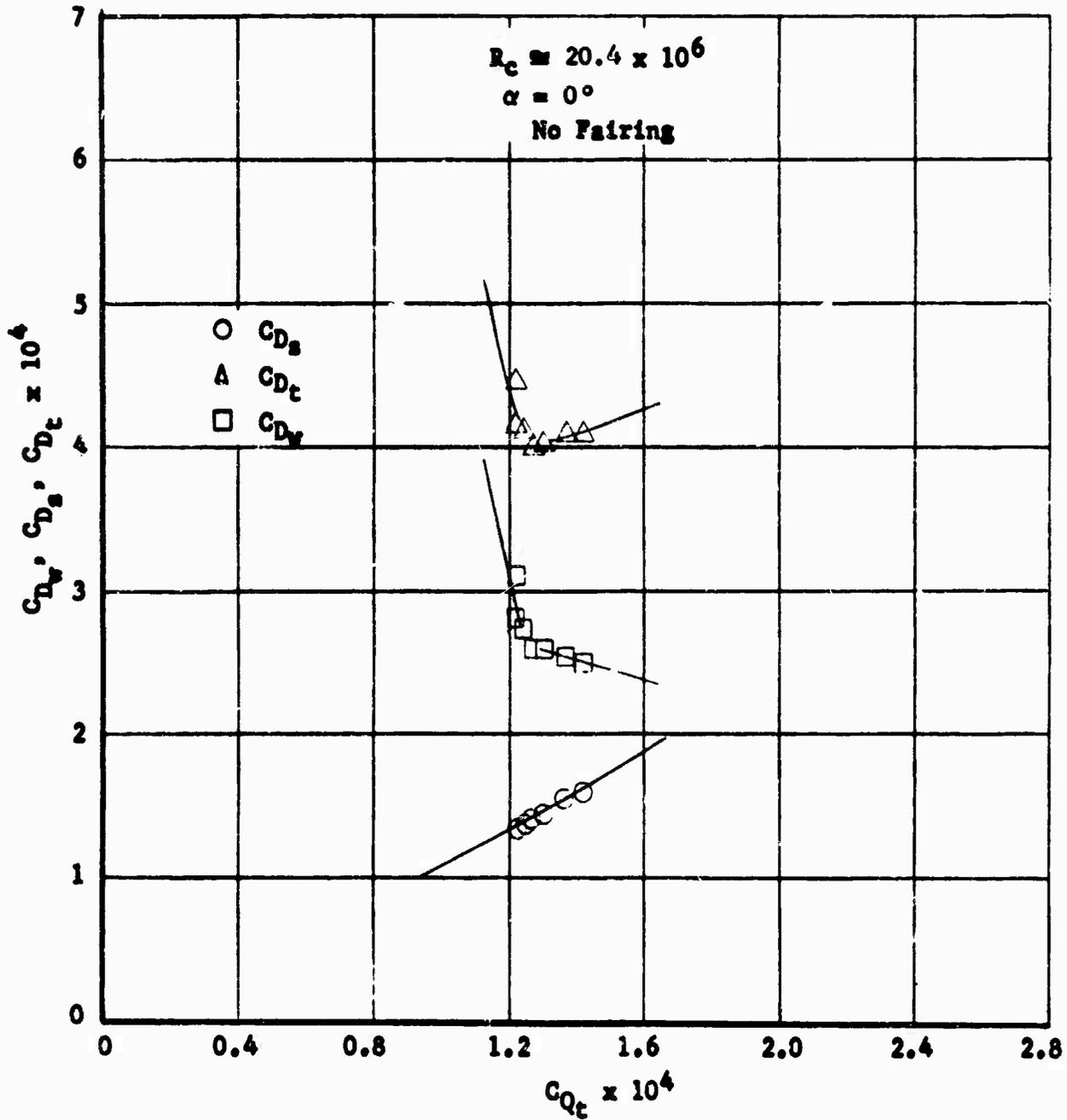
FIGURE 36 DRAG  $C_D$  VERSUS SUCTION QUANTITY  $C_{Q_t}$  FOR VARIOUS REYNOLDS NUMBERS  $R_c$  AND ANGLES OF ATTACK  $\alpha$
