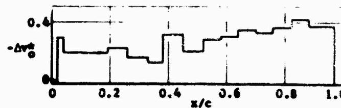
FIGURE 76 ADDITIONAL SUCTION  $-\Delta v^2$ , REQUIRED TO MAINTAIN LAMINAR FLOW AT VARIOUS FREQUENCIES AND EXTERNAL SOUND PRESSURE LEVELS,  $R_c = 20.2 \times 10^6$
