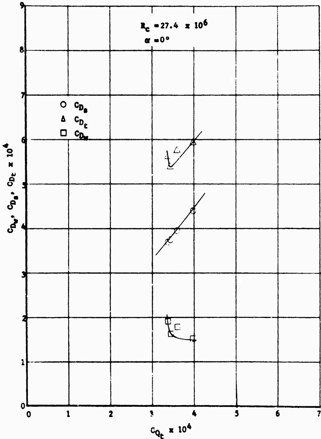
FIGURE 6 DRAG  $C_D$  VERSUS SUCTION QUANTITY  $C_{Qt}$  FOR VARIOUS REYNOLDS NUMBERS  $R_c$  AND ANGLES OF ATTACK  $\alpha$
