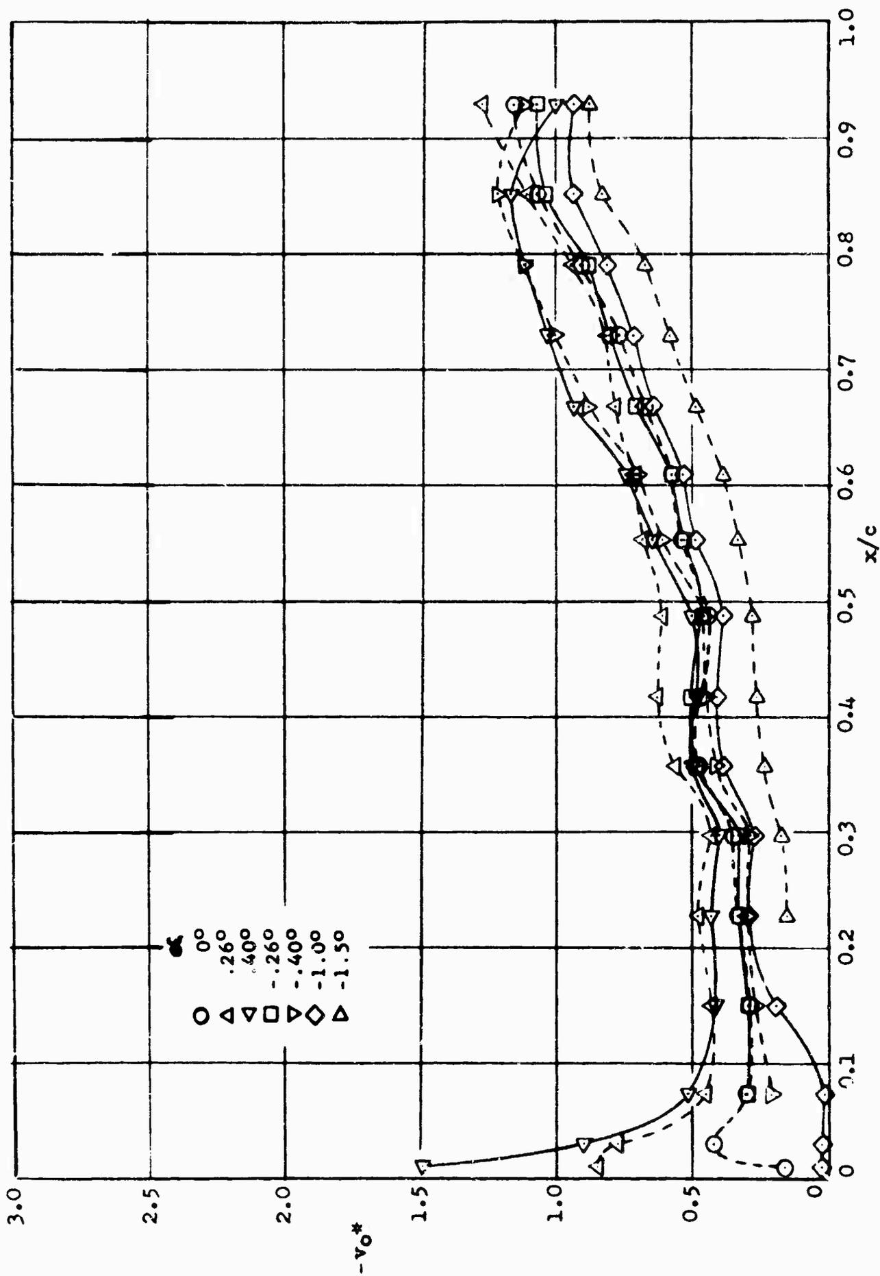
FIGURE 52 NONDIMENSIONAL EQUIVALENT AREA SUCTION VELOCITY  $v_0^*$  DISTRIBUTION NEAR OPTIMUM SUCTION COEFFICIENT  $C_{Q_{opt}}$  FOR SEVERAL ANGLES OF ATTACK  $\alpha$  AT A REYNOLDS NUMBER  $R_c$  OF APPROXIMATELY  $21 \times 10^6$
