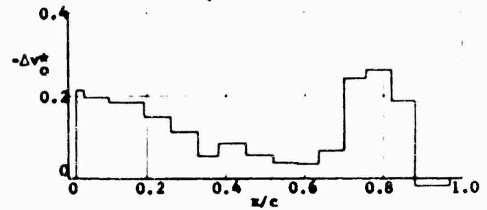
FIGURE 77 ADDITIONAL SUCTION,  $-\Delta v_0^*$ , REQUIRED TO MAINTAIN LAMINAR FLOW AT VARIOUS FREQUENCIES AND EXTERNAL SOUND PRESSURE LEVELS,  $R_c = 21.5 \times 10^6$
