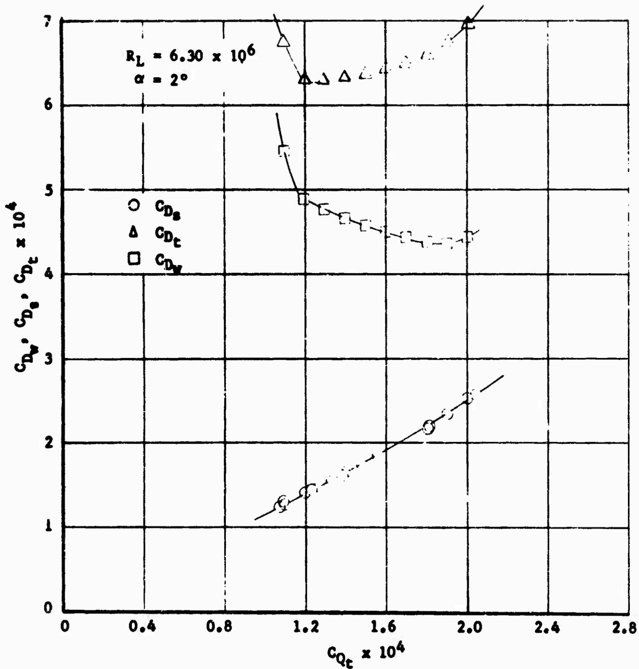
FIGURE 180 DRAG  $C_D$  VERSUS SUCTION QUANTITY  $C_{Qc}$  FOR VARIOUS REYNOLDS NUMBERS  $R_c$  AND ANGLES OF ATTACK  $\alpha$
