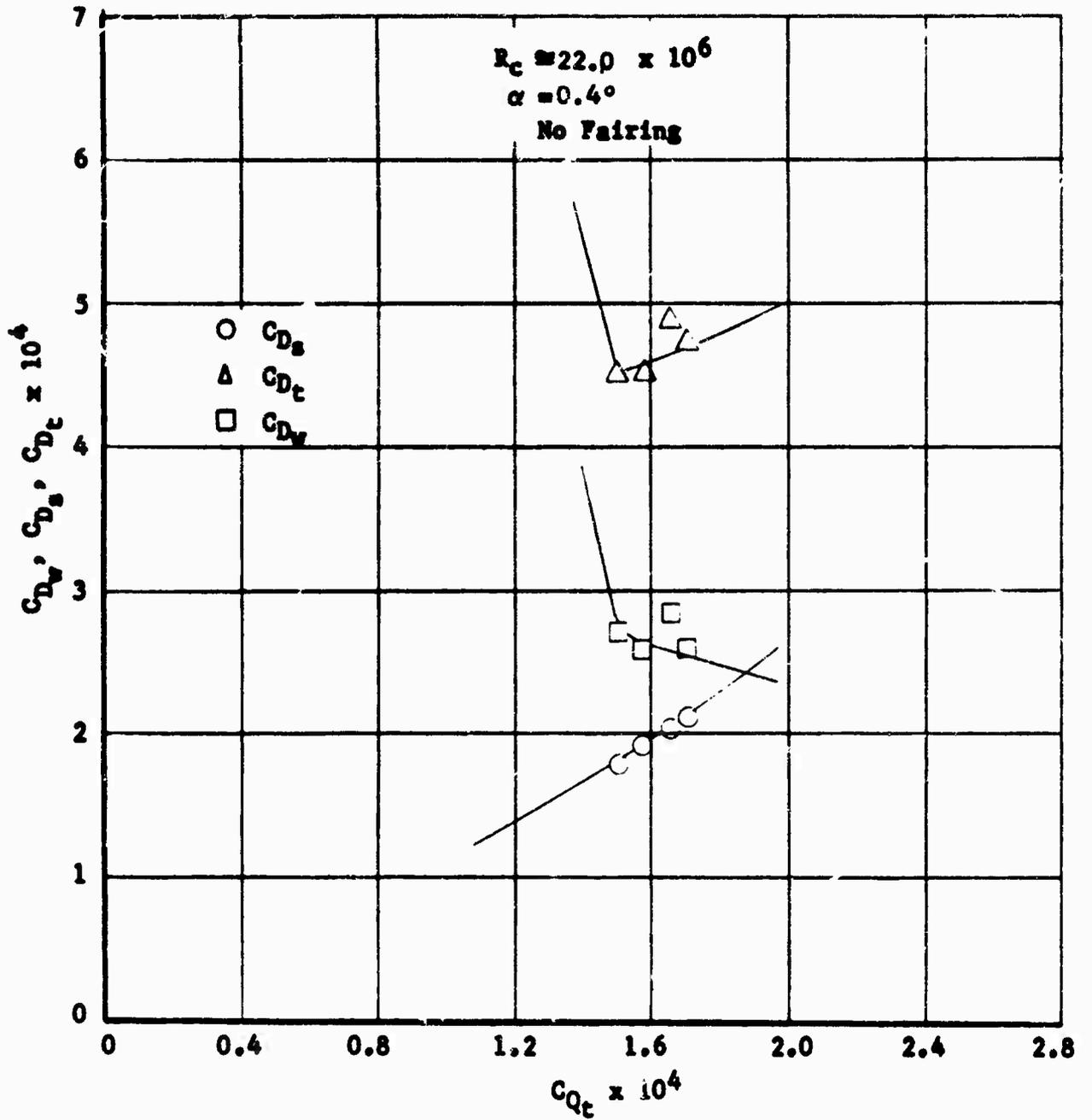
FIGURE 38 DRAG  $C_D$  VERSUS SUCTION QUANTITY  $C_{Q_c}$  FOR VARIOUS REYNOLDS NUMBERS  $R_c$  AND ANGLES OF ATTACK  $\alpha$
