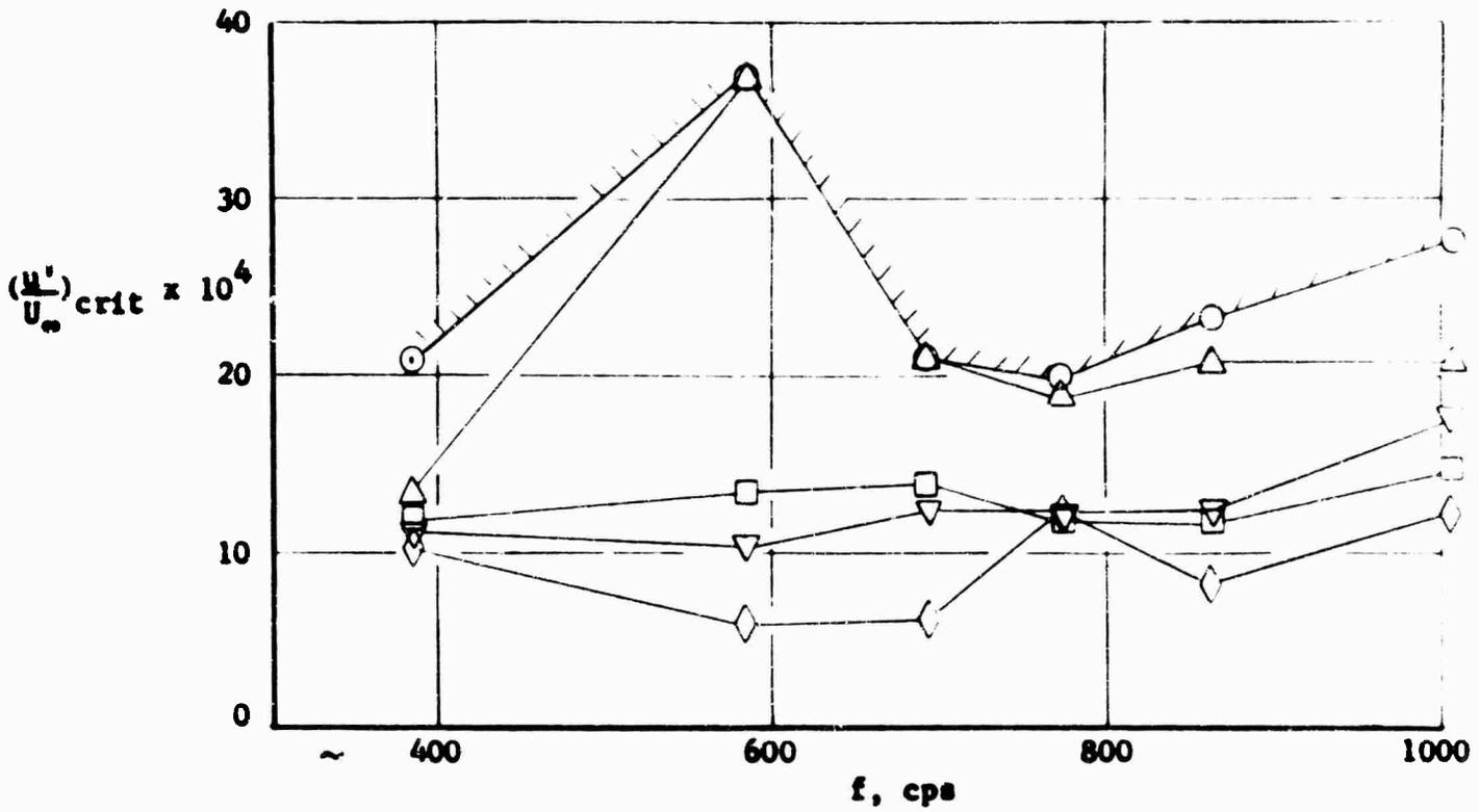
**FIGURE 137** EXTERNAL SOUND LEVEL TO CAUSE TRANSITION AS A FUNCTION OF FREQUENCY,  $R_c = 14.2 \times 10^6$
