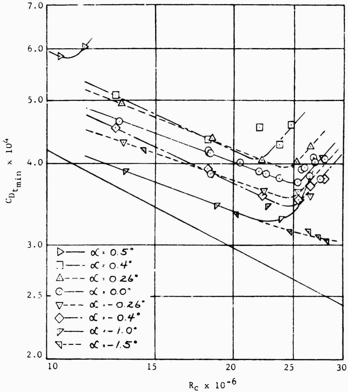
FIGURE 43 VARIATION OF MINIMUM TOTAL DRAG COEFFICIENT  $C_{Dt}$  (INCLUDING EQUIVALENT SUCTION DRAG) WITH REYNOLDS NUMBER  $R_c$  FOR SEVERAL ANGLES OF ATTACK  $\alpha$
