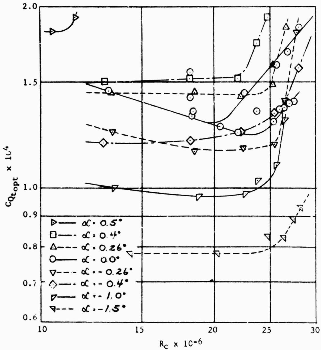
FIGURE 44 VARIATION OF OPTIMUM SUCTION COEFFICIENT  $C_{Qt_{opt}}$  WITH REYNOLDS NUMBER  $R_c$  FOR SEVERAL ANGLES OF ATTACK  $\alpha$
