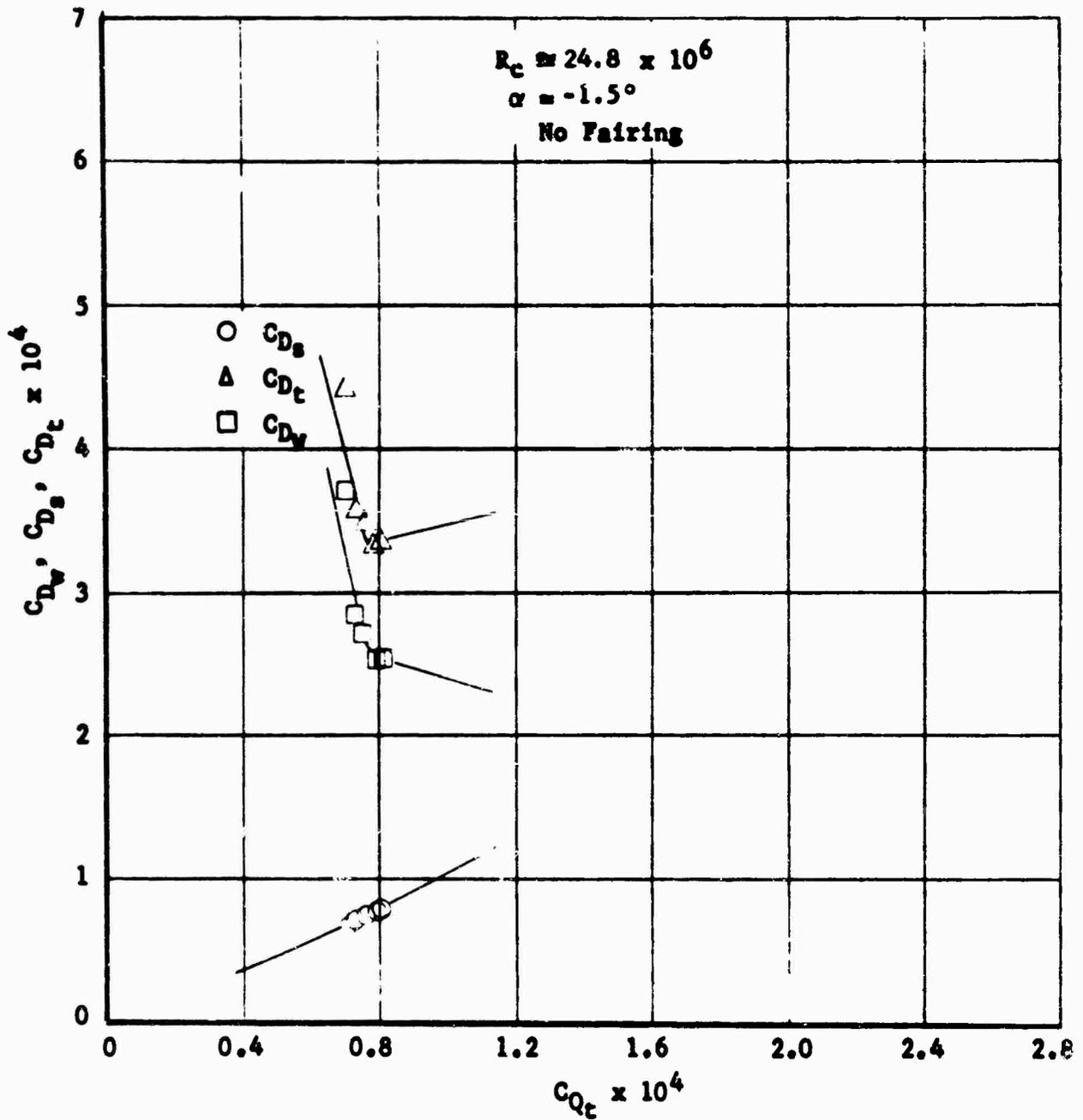
FIGURE 42 DRAG  $C_D$  VERSUS SUCTION QUANTITY  $C_{Q_t}$  FOR VARIOUS REYNOLDS NUMBERS  $R_c$  AND ANGLES OF ATTACK  $\alpha$
