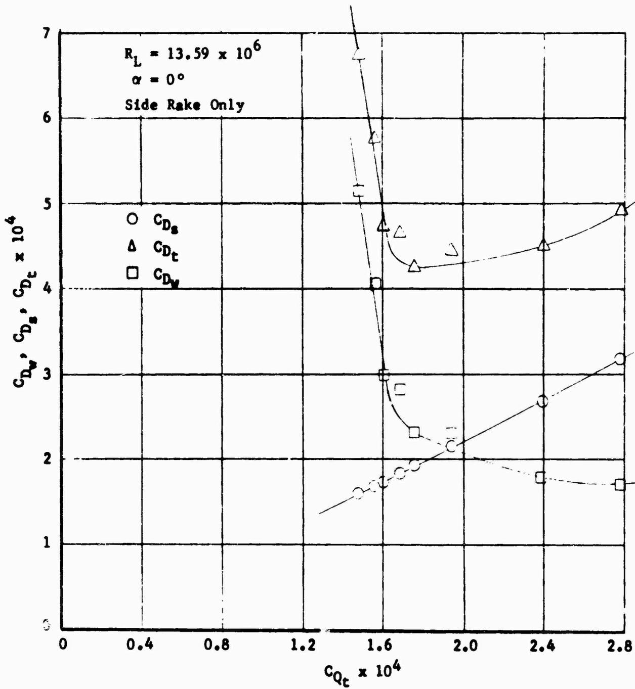
FIGURE 175 DRAG  $C_D$  VERSUS SUCTION QUANTITY  $C_{Q_c}$  FOR VARIOUS REYNOLDS NUMBERS  $R_c$  AND ANGLES OF ATTACK  $\alpha$
