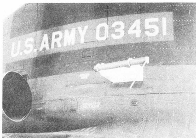
FIGURE 25: EXHAUST PROBE INSTALLATION ON CH-47A AIRCRAFT
