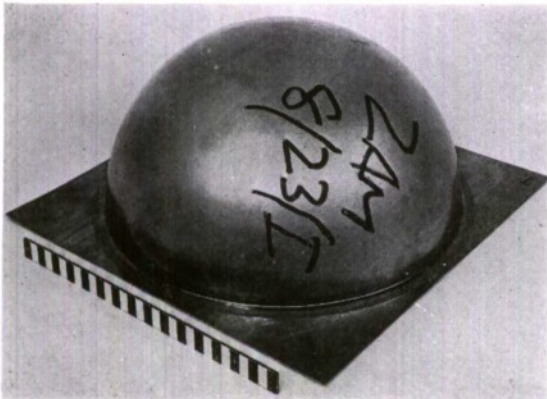
FIG. 4. First hemisphere formed from ZAM sheet
