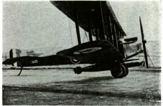
FIG. 23. Torpedo-Carrying aeroplane, Sopwith (T) carrying 18 in. Mark IX with heavy head (250 lbs. explosives).
