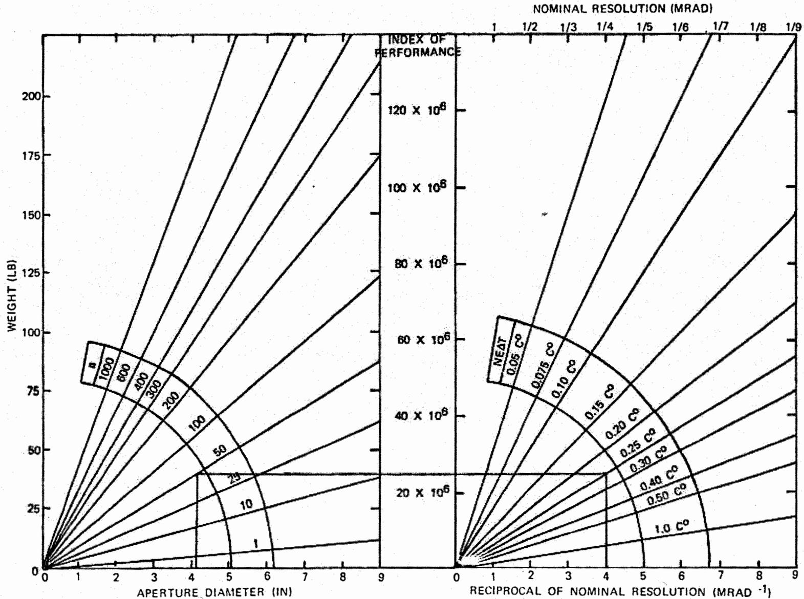
FIGURE 2 - Nomograph of FLIR Tradeoffs (U)
