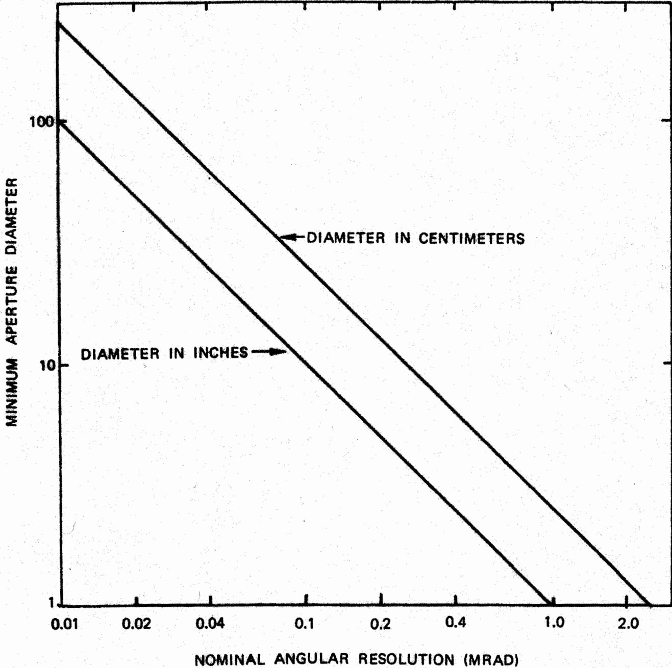
FIGURE 3 - Minimum Aperture Diameter For a Diffraction Limited FLIR as a Function of Required Resolution (U)
