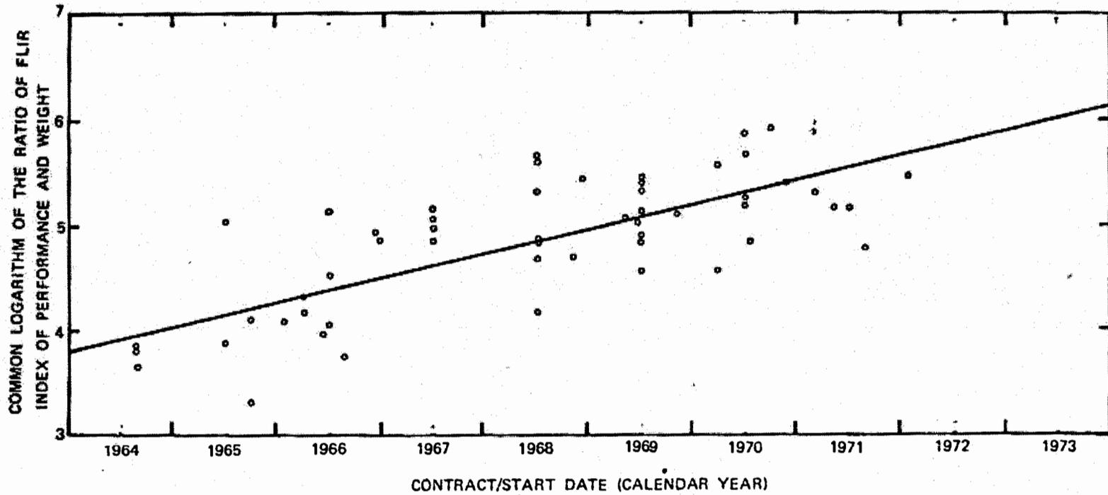
FIGURE 4 - FLIR Performance-to-Weight Ratios as a Function of Contract/Start Date (U)
