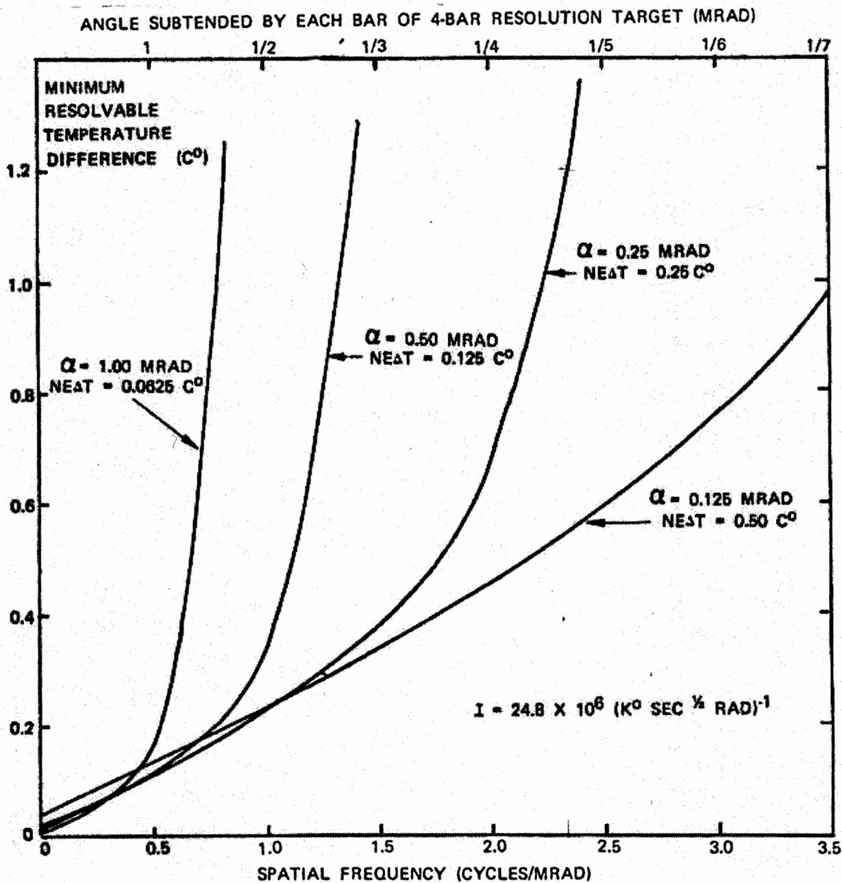
FIGURE 5 - Family of MRT Curves for Four Hypothetical FLIRs Having Equal Indices of Performance (U)
