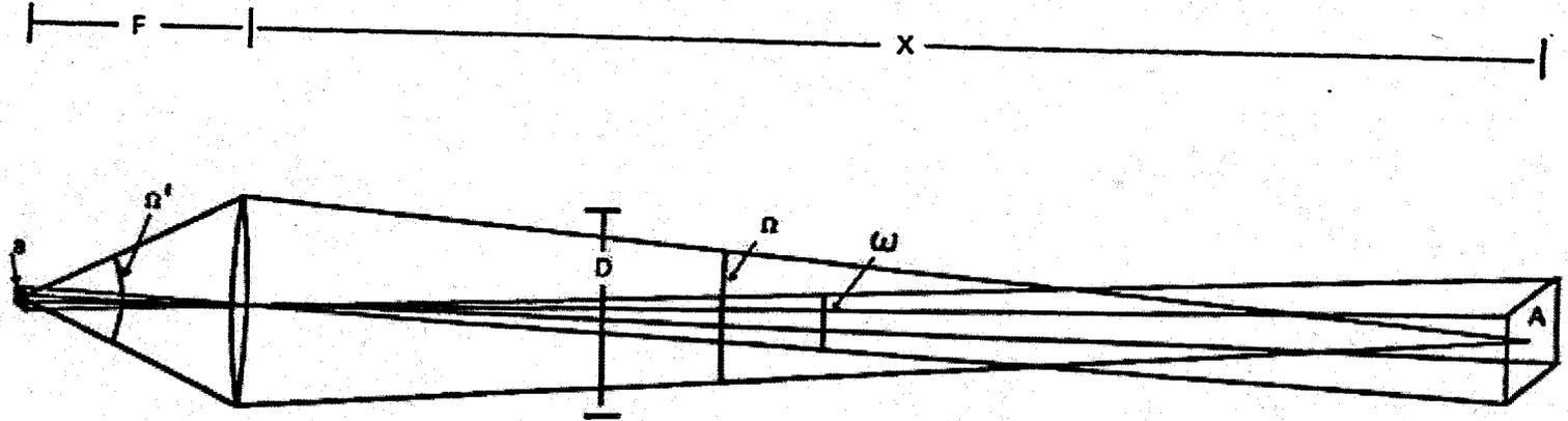
FIGURE 1 - Description of Geometrical Terms Used in Derivation of FLIR Performance Equations (U)
